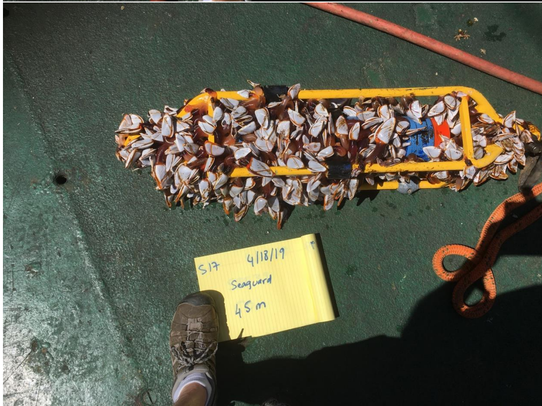
Figure III-4. Heavy biofouling on instrumentation in the upper 50 m.
