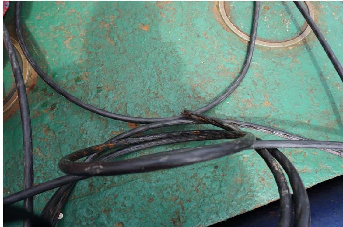
Figure III-3. Break of the Stratus 17 mooring line, a few meters below a VMCM. The plastic jacket shows signs of abrasions for several meters, exposing the wire inside to corrosion.
