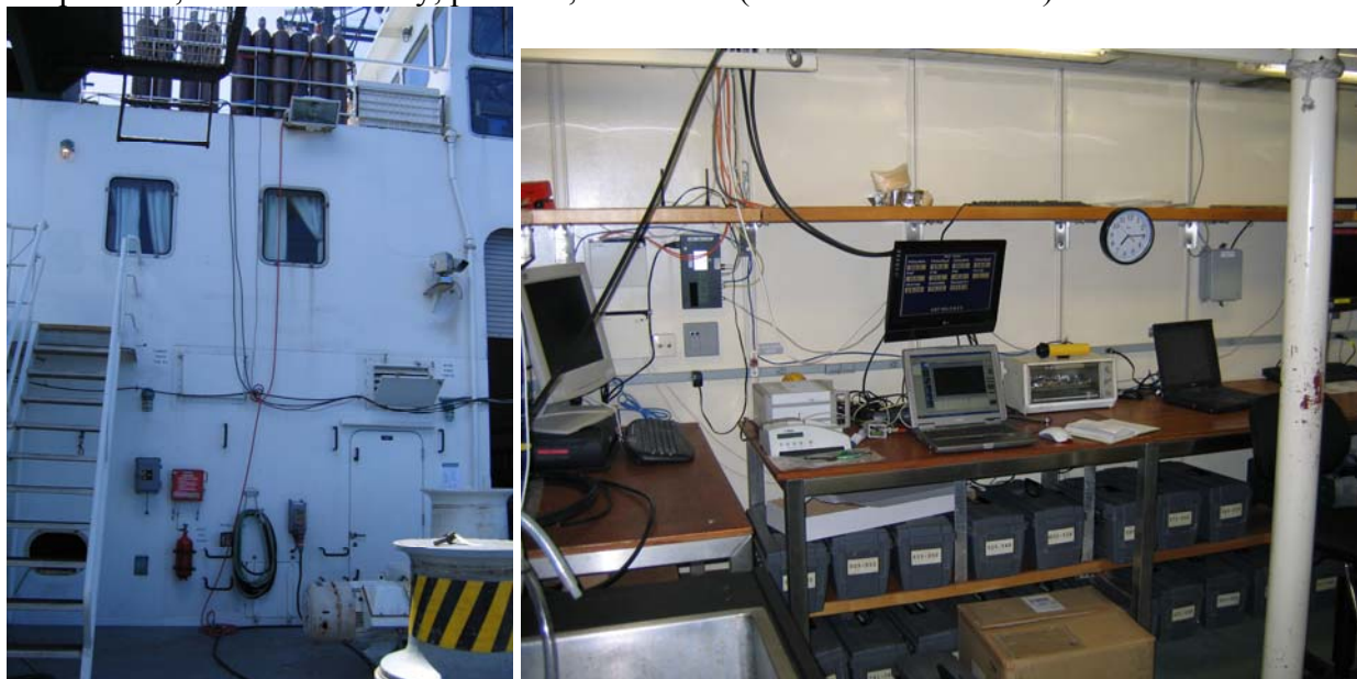
Figure 10-5: Left panel: view of the inflation site on the main deck with the Helium bottles on the 02 deck. Right panel: Vaisala radiosonde system deployed in Lab#1 of the Main deck.
