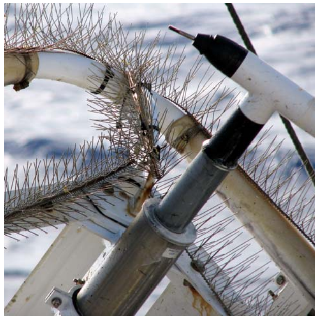
Figure 5-5. WHOTS-5 WND module SN 205 after buoy recovery. Missing propeller and bent shaft are evident. Note also the near proximity of anti-bird wire to the module housing.
