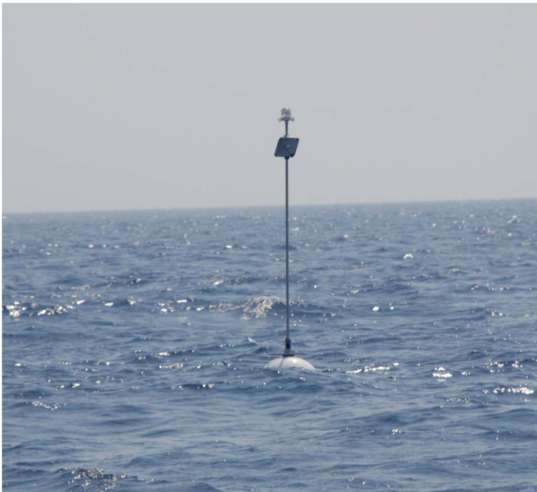
Figure 11: The surface buoy of the reef-edge mooring, showing the light and radar reflector at the top of the buoy mast.
