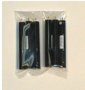
Batteries packed for shipment by commercial aircraft
