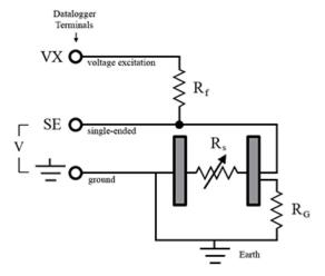
With R<sub>g</sub> in the resistor network, the signal measured from the sensor is described by the following equation:
