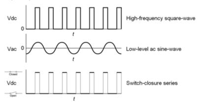
Pulse input terminals and the input types they can measure
