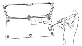
6. Reassemble the datalogger. Take particular care to ensure the canister is reseated tightly into the connectors by firmly pressing them together by hand.
