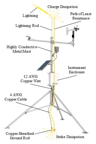
All critical inputs and outputs on the datalogger are ESD protected to 75 V. To be effective, the earth ground lug must be properly connected to earth (chassis) ground.
