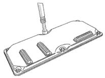
5. Remove the lithium battery by gently prying it out with a small slot head screwdriver.
