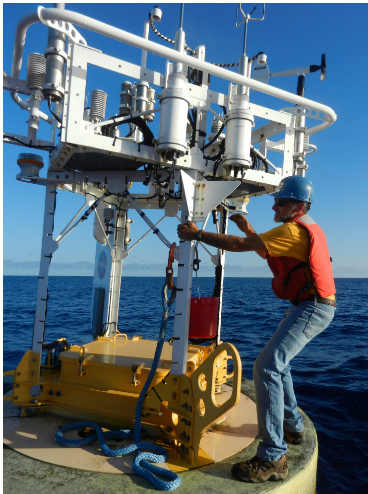
Figure 5.2 Jeff Lord attaches pickup sling to WHOI buoy.
