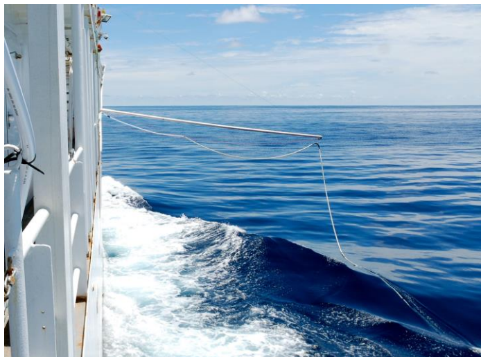
Figure K1: Salinity Snake Mk. 2 Intake system, showing mast and vacuum rated EPDM/nylon/steel hose with intakes and recording thermistor acting as hose stopper.
