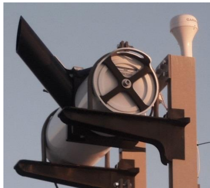
Figure J1: ROSR with rain baffle.
