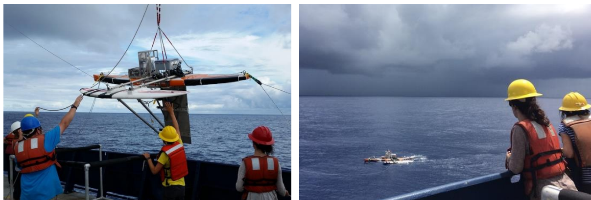
Figure I1: Left image: The Surface Salinity Profiler (SSP) used during the 2016 SPURS2 field experiment being deployed from the R/V Revelle . Right image: The SSP under tow.
