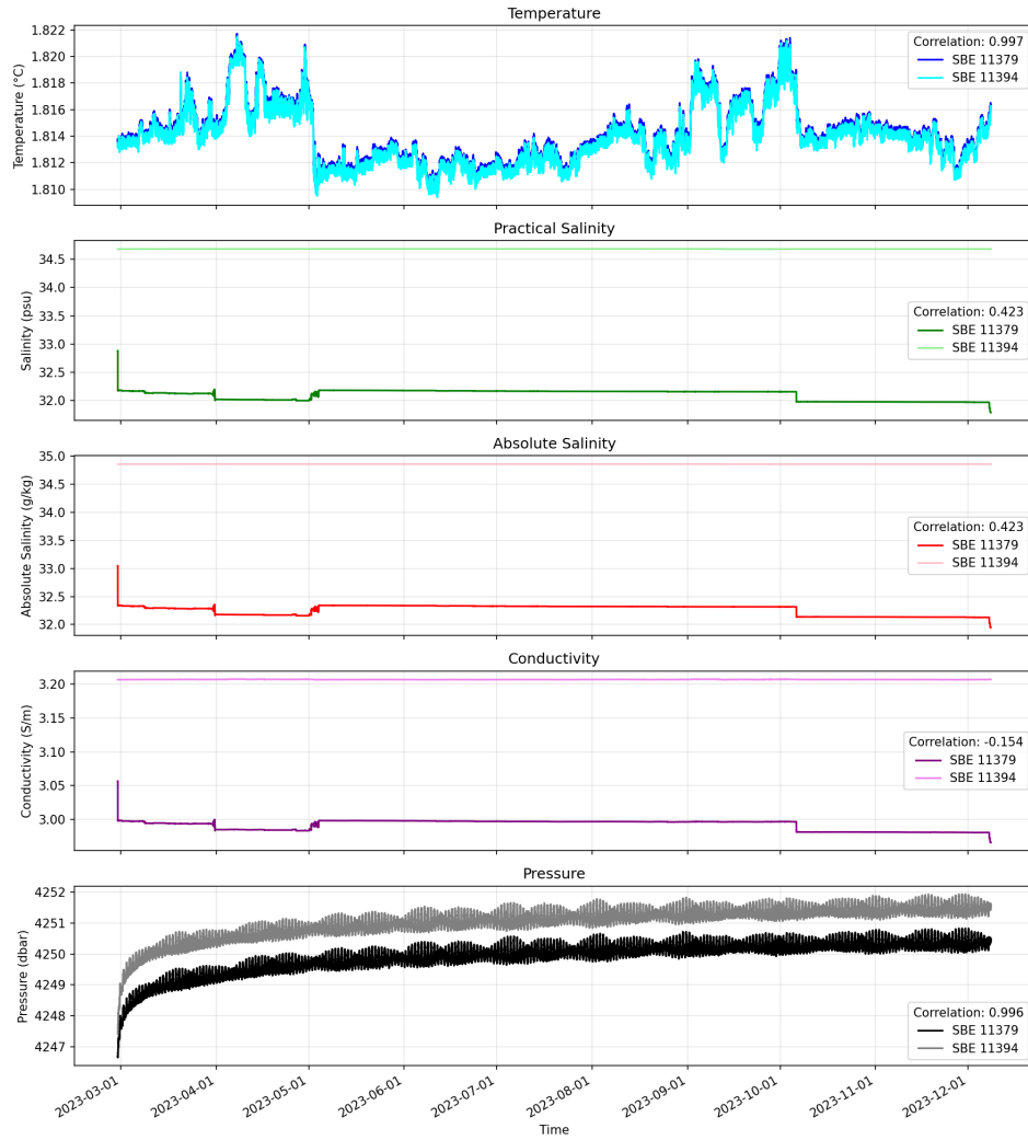
Figure 5: Deployment and recovery timing analysis for stratus 21, comparing instruments SBE37 11379 and SBE37 11394. This figure shows the expected time window of good data after truncation. Truncated dataset starts 4 hours after anchor over time and ends at release fired time.
