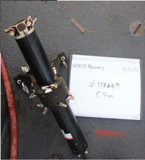
Figure IV-10. NTAS19: Nortek current meters and profilers.
