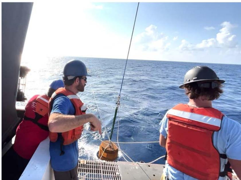
**Figure III-8. NTAS 20 surface mooring anchor just before release**
