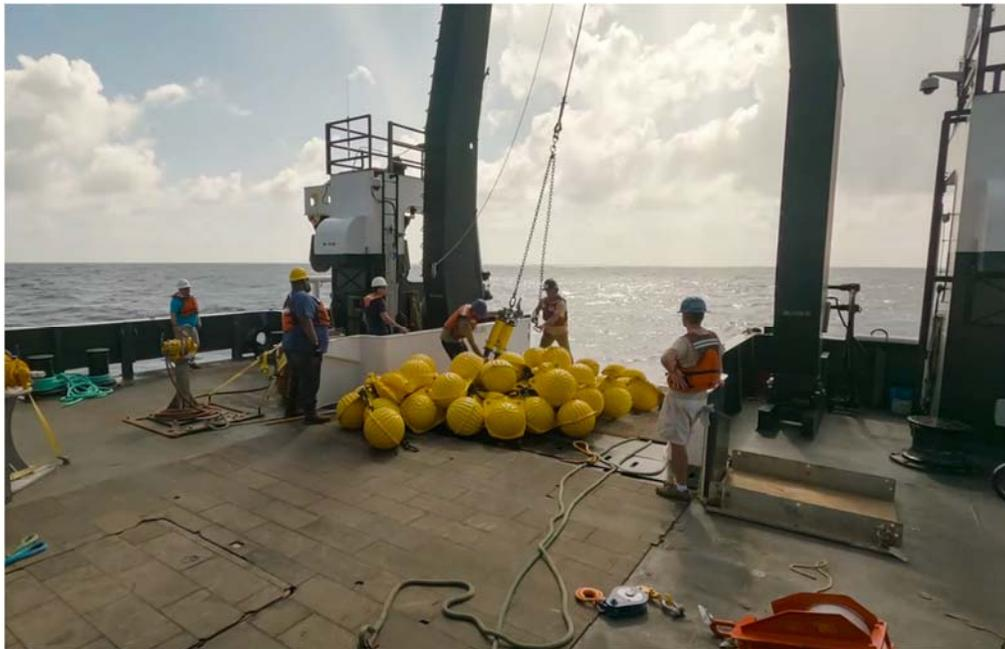
**Figure IV-2. Recovery of the NTAS 19 dual acoustic releases with cluster of glass ball floats on deck.**
