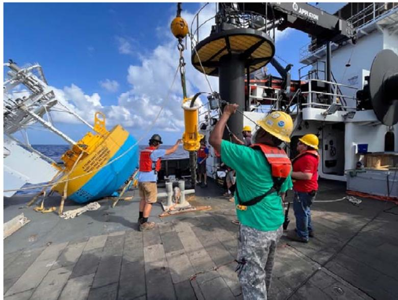
Figure III-4. Subsurface telemetry system being deployed over the port side of the NOAA F/V *Pisces*.
