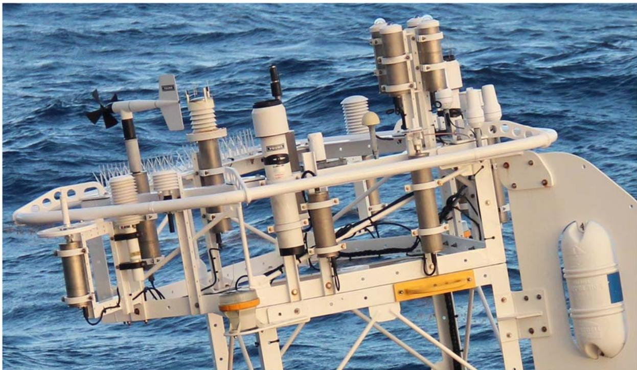
**Figure IV-5. ASIMET meteorological sensors immediately prior to recovery of NTAS19.**
