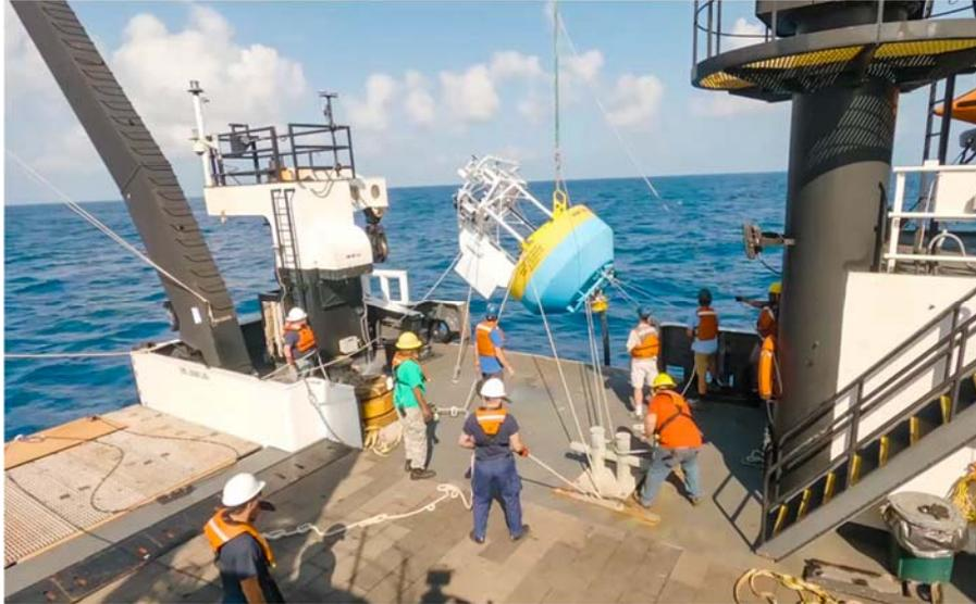
**Figure III-6. NTAS 20 Surface buoy deployment over the port side of the NOAA F/V Pisces**
