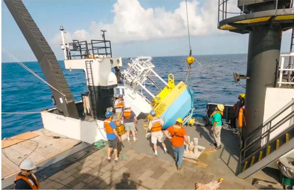
**Figure III-5. Preparing the NTAS 20 surface buoy for deployment with EM chain deployed over the port side.**
