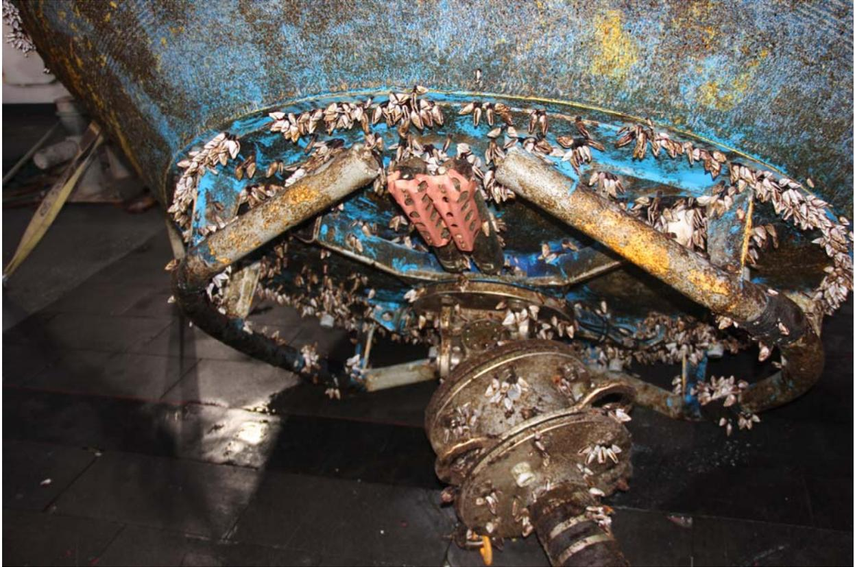
**Figure IV-6. NTAS 19 buoy bridle immediately following recovery.**
