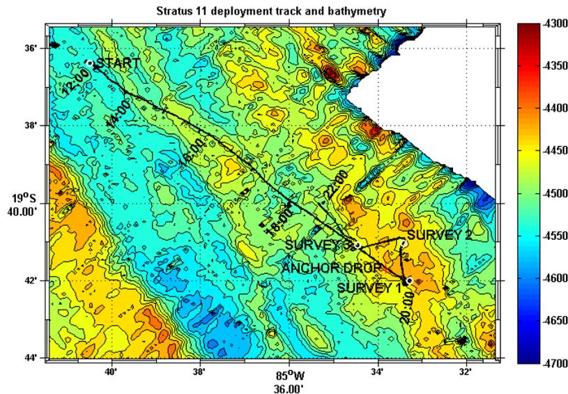
**Figure 3-5.** Stratus 11 deployment track on April 6 2011. Start of track is about 8 nm downwind of target anchor drop. Three anchor survey points are shown too. Time (UTC) of day is indicated along track. Color contours are bathymetry (in m; contour interval 20m) from Seabeam data (not corrected for speed of sound or transducer depth; correction should be +10m) collected during Stratus 9 cruise.
