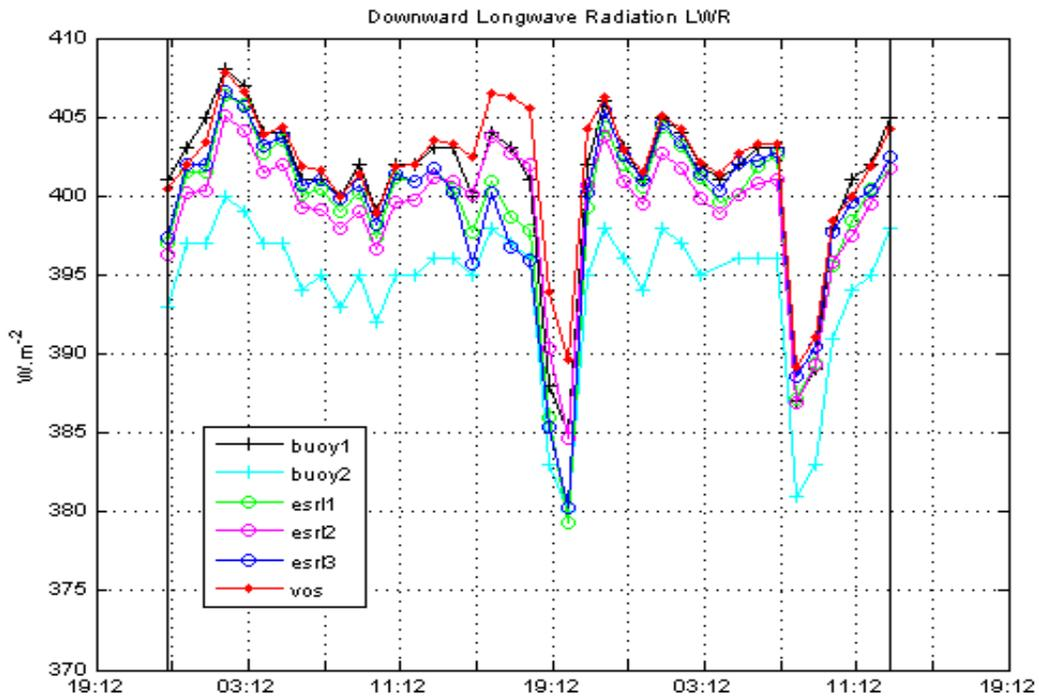
**Figure 3-16.** Downward LWR on during Stratus 11 deployment intercomparison. ESRL sensors 1 to 3 are Eppley above bridge, Kipp & Zonen on bridge, and Eppley on O2 deck, respectively. VOS is Eppley above bridge. Vertical black lines denote start and end of intercomparison period.
