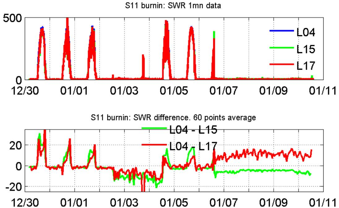
**Figure 2-1.** Last burn-in period in WHOI when buoy was outside. Upper panel shows time-series from 1-minute downward shortwave solar radiation (SWR) data, in  $\text{Wm}^{-2}$ . Lower panel shows the difference between sensors, averaged over 1 hour.
