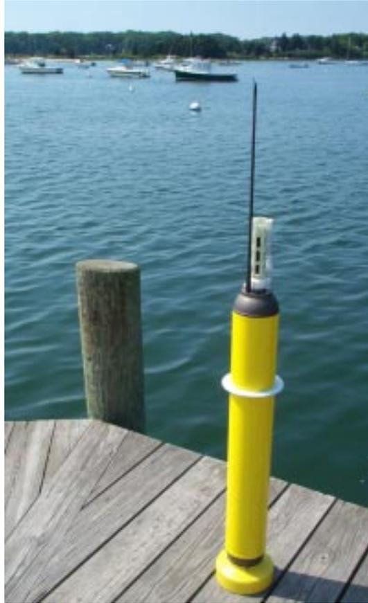
**Figure 5-8.** Apex Float of the type deployed during stratus 11 cruise.
