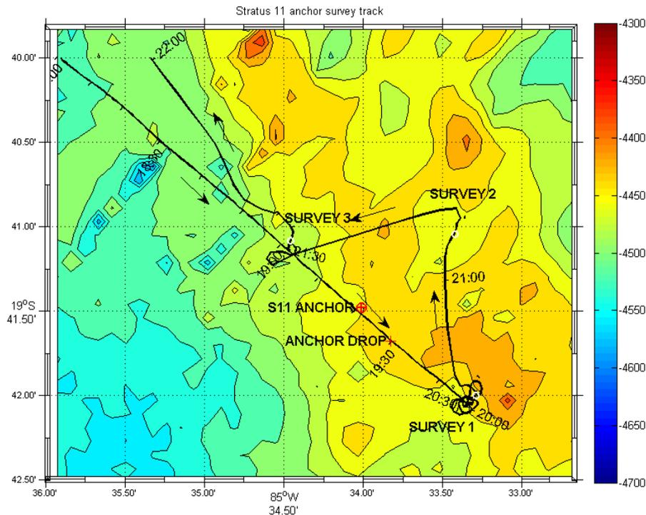
**Figure 3-6.** Stratus 11 deployment track. Same as Fig. 3-5 but Seabeam data is corrected for speed of sound (+5m) and transducer depth (+5m). Stratus 11 anchor location on seafloor indicated by red circle with cross. Depth at anchor location is 4440m.
