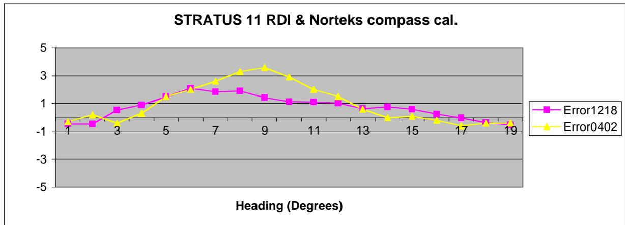
**Figure 3-4.** Compass error from ADCPs RDI Workhorse Sentinel (SN 1218, deployed at 135m depth) and Nortek (SN 357 deployed at 10m), deployed on Stratus 11. Note that there is a mistake in the legend: the Nortek serial number is 357, not 402.
