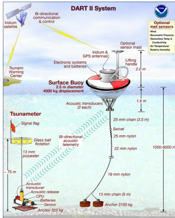
**Figure 5-11.** Schematic of the DART mooring system.
