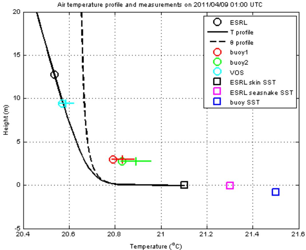
**Figure 3-20.** Air temperature measured on ship and buoy. Vertical profile from COARE 3.0 in black (dashed line is potential temperature), using hourly averaged value for time 01:00 UTC on 04/09/2011 (night time). Measurements at this hour are denoted by circles or squares. Small vertical bars indicate the average distance between the profile and measurements over the last 24 hours of the intercomparison, whereas the horizontal lines denote its standard deviation.
