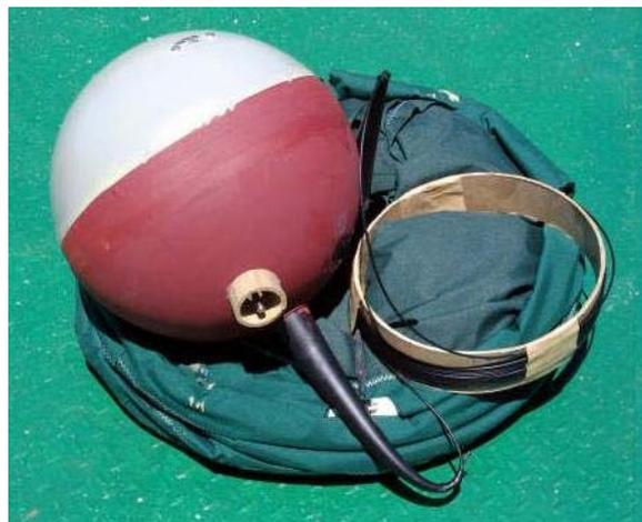
**Figure 5-9.** Typical Surface Drifter
