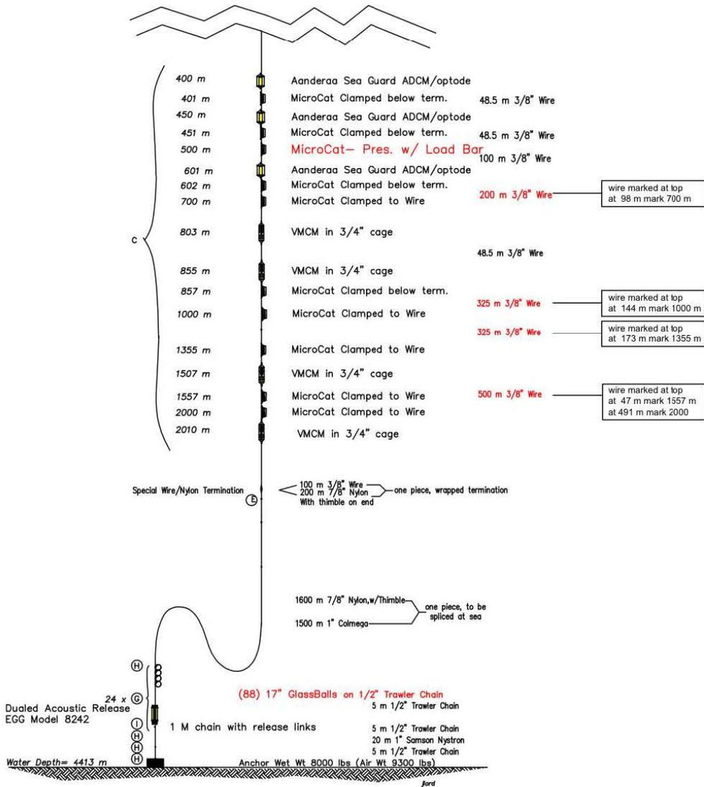
Figure 3-2. Stratus 11 mooring diagram (bottom part).
