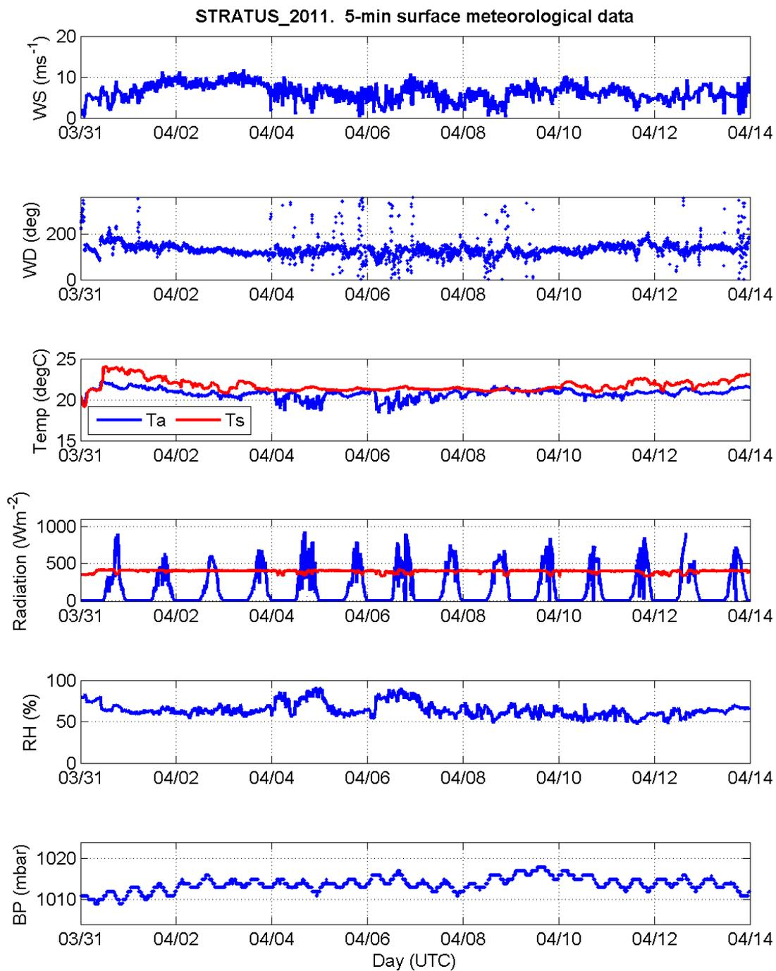
**Figure 3-11 (part 2).** Time series of the surface meteorological data collected during the Stratus 11 cruise.
