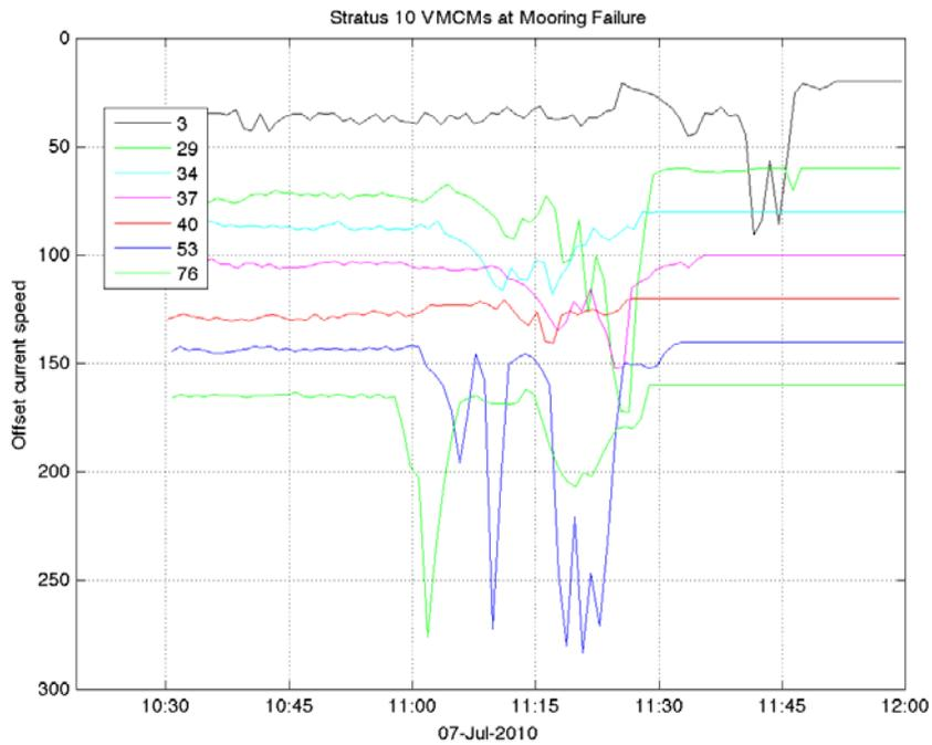
**Figure 4-7.** Stratus 10 VMCMs at time of mooring failure.
