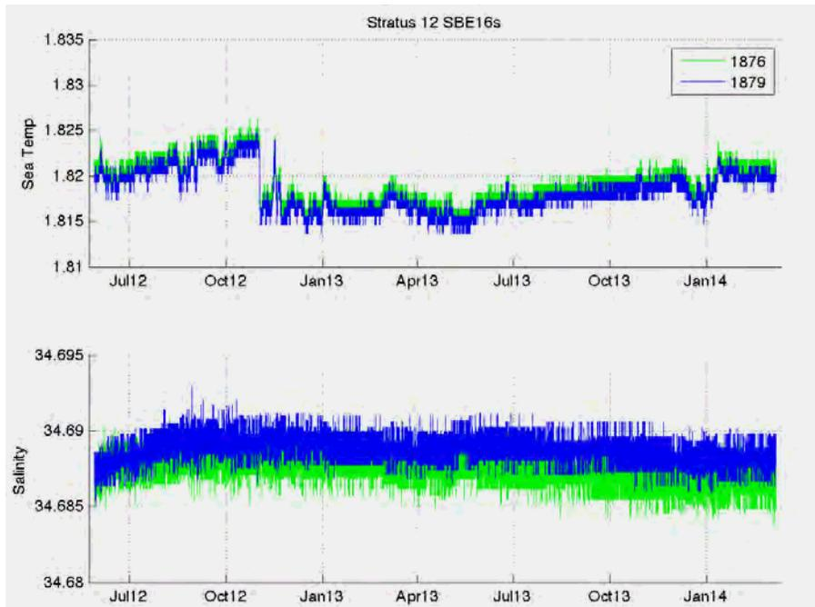
Figure 4-10. Temperature and salinity records from deep SBE16s on the Stratus 12 mooring.
