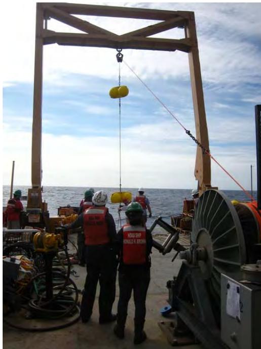
**Figure 5-3.** Recovering the existing NDBC BPR mooring.
