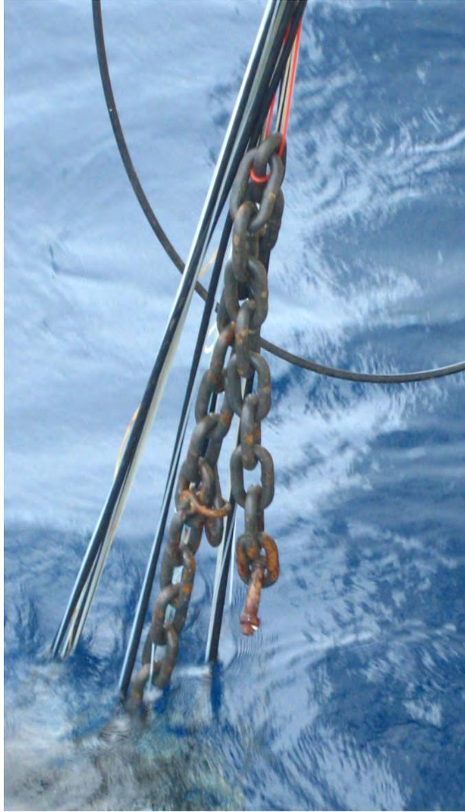
**Figure 4-7.** The end of a chain with a pin and cotter pin but no shackle, seen during the recovery of Stratus 12 mooring which had fallen to the ocean floor (see also Fig. 4-6).
