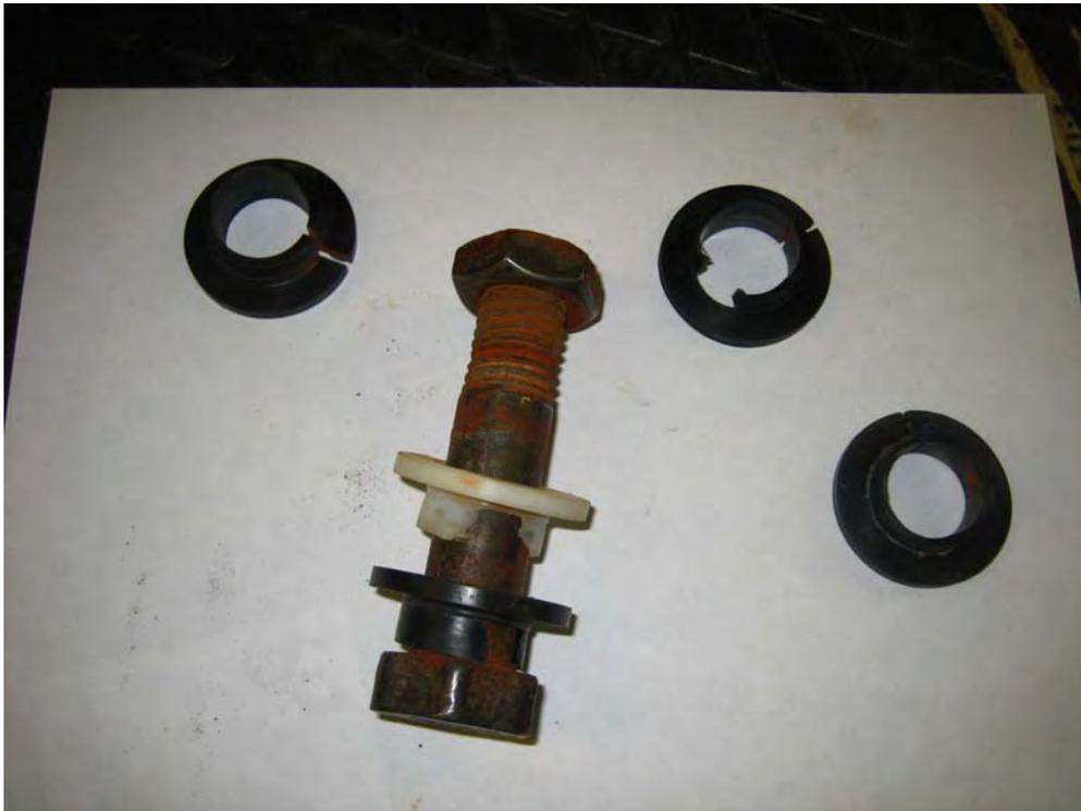
**Figure 4-2.** Hardware near the failure point under the recovered Stratus 12 buoy. Bushings that were isolating titanium load bars from shackles are worn out and zinc coating on pins and shackles is gone.
