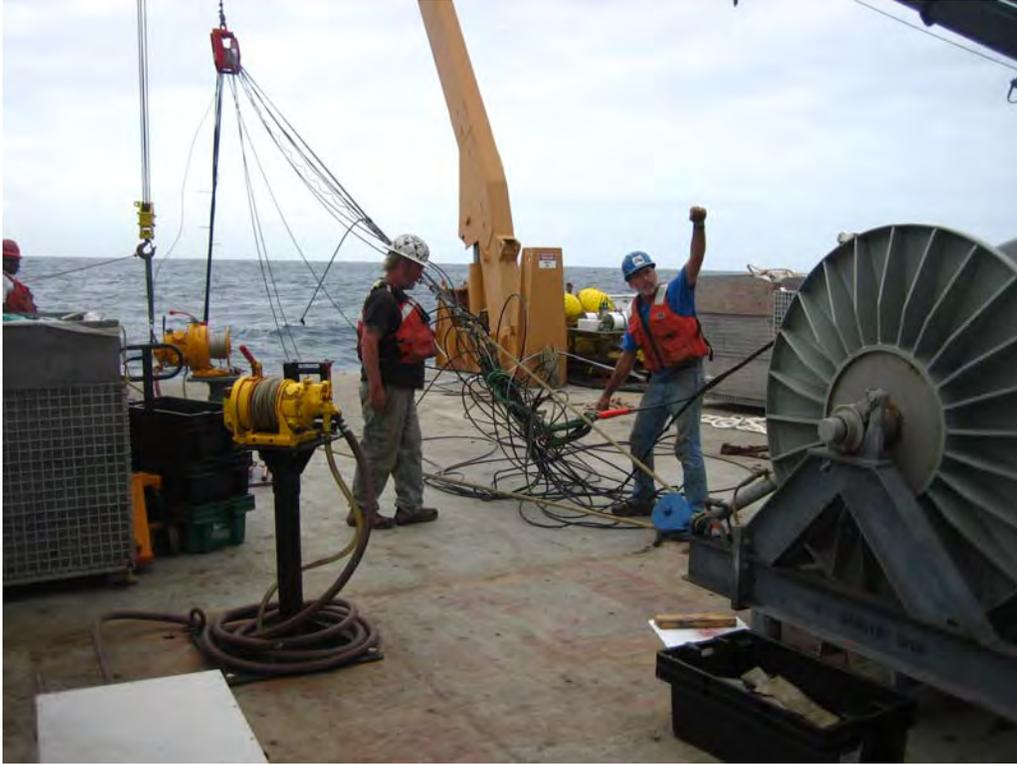
**Figure 4-3.** Stratus 12 recovery: tangle of wire with one end tied to the TSE winch and wire clamps connected to stop line to check which wire holds tension and cut the others.
