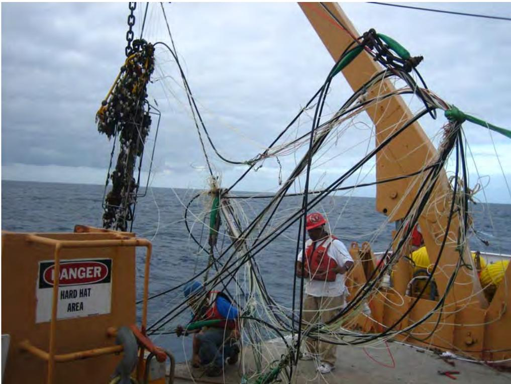
**Figure 4-4.** Stratus 12 recovery: wire and instruments from Stratus 12 mooring after it fell to the bottom. Fishing gear fouling is heavy.
