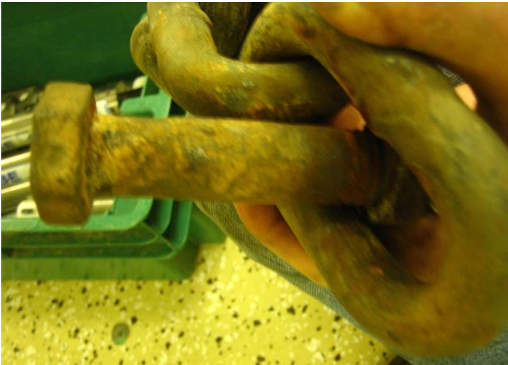
**Figure 4-6.** The failed part of mooring Stratus 12 (see also Fig. 4-7). ""
