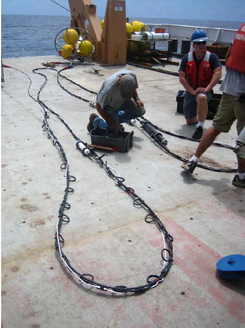
**Figure 5-9.** Mini-array laying out on deck before deployment. Note the surface frame with three flotation glass balls (top center), which also holds two XR420 loggers. 12 m further down the line are the next two similar loggers and a DR-150 pressure sensor, with one Nortek profiler above and one below them. Another 12 m is the last XR420 logger and the last instrument is the second DR-150 (top left).
