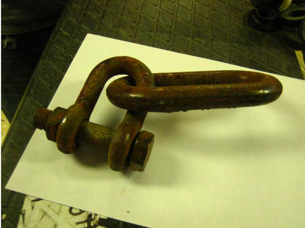
**Figure 4-1.** Bottom part of remaining mooring line under the drifting Stratus 12 buoy. Only a link left with no shackle below. The shackle seen here is the one above, which was attached to the instrument above.
