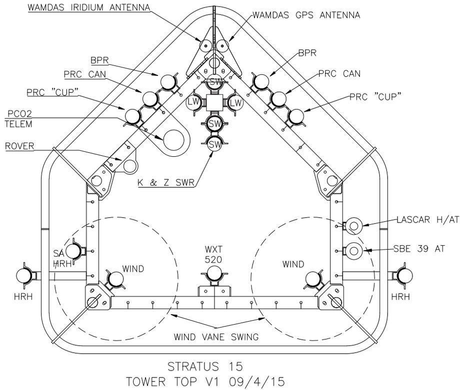
**Figure III-1. Top view schematic of the meteorological tower on the STRATUS 15 buoy with the location of the ASIMET and other instruments.**
