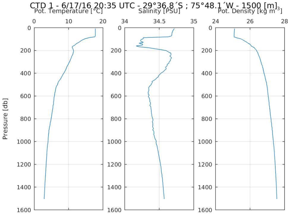
**Figure V-1. CTD profile data collected on June 17 2016, for acoustic releases test.**
