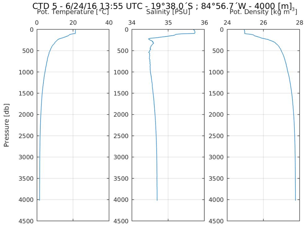
**Figure V-9. CTD profile data collected on June 24 2016, near the Stratus 15 buoy.**
