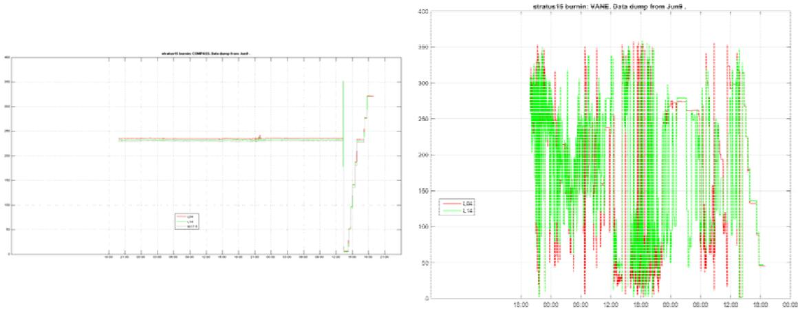
**Figure II-2. One-minute data from STRATUS 15 buoy spin on June 9 2016: compass (left) and wind sensor vane (right).**
