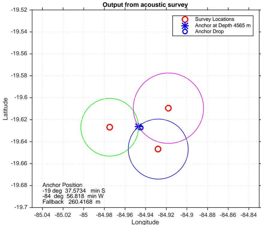
**Figure III-7. Anchor survey results using Anchpos code from Weller.**
