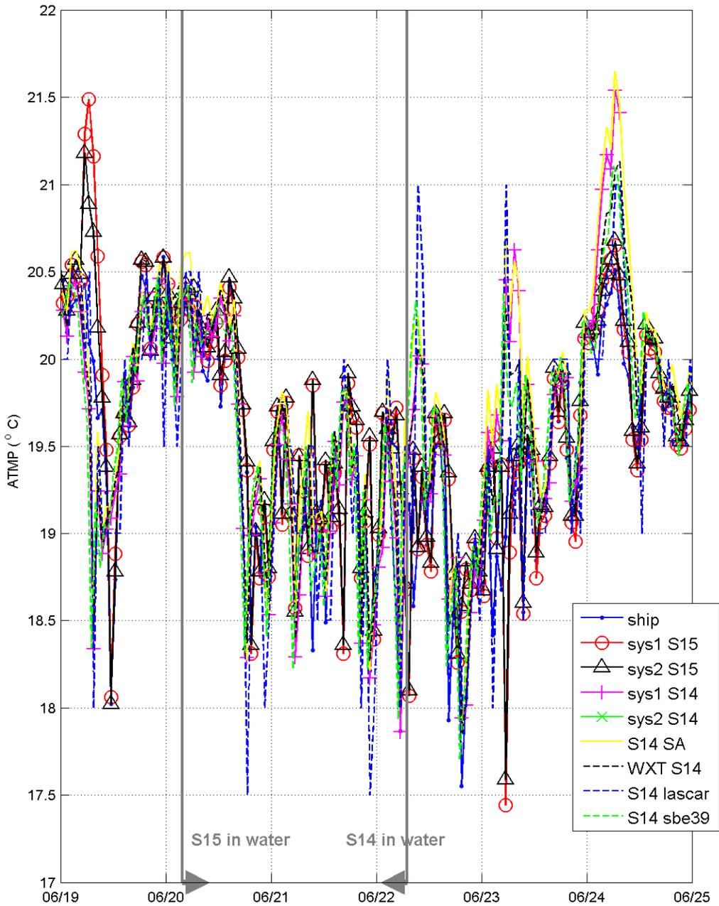
Figure III-8. Inter-comparison between Stratus 14 and 15 buoys and sensors on ship: air temperature (ATMP).
