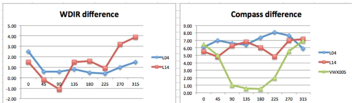
**Figure II-1. STRATUS 15 buoy spin on April 21 2016 in Woods Hole. Y-axis: difference between wind direction (L04 and L14), or compass (WXT005), and line-of-sight reference (in degrees). X-axis: angle between buoy and line-of-sight reference (in degrees). Note that operator reoriented the WXT during Turn=90, by small angle (~ 10 degrees).**
