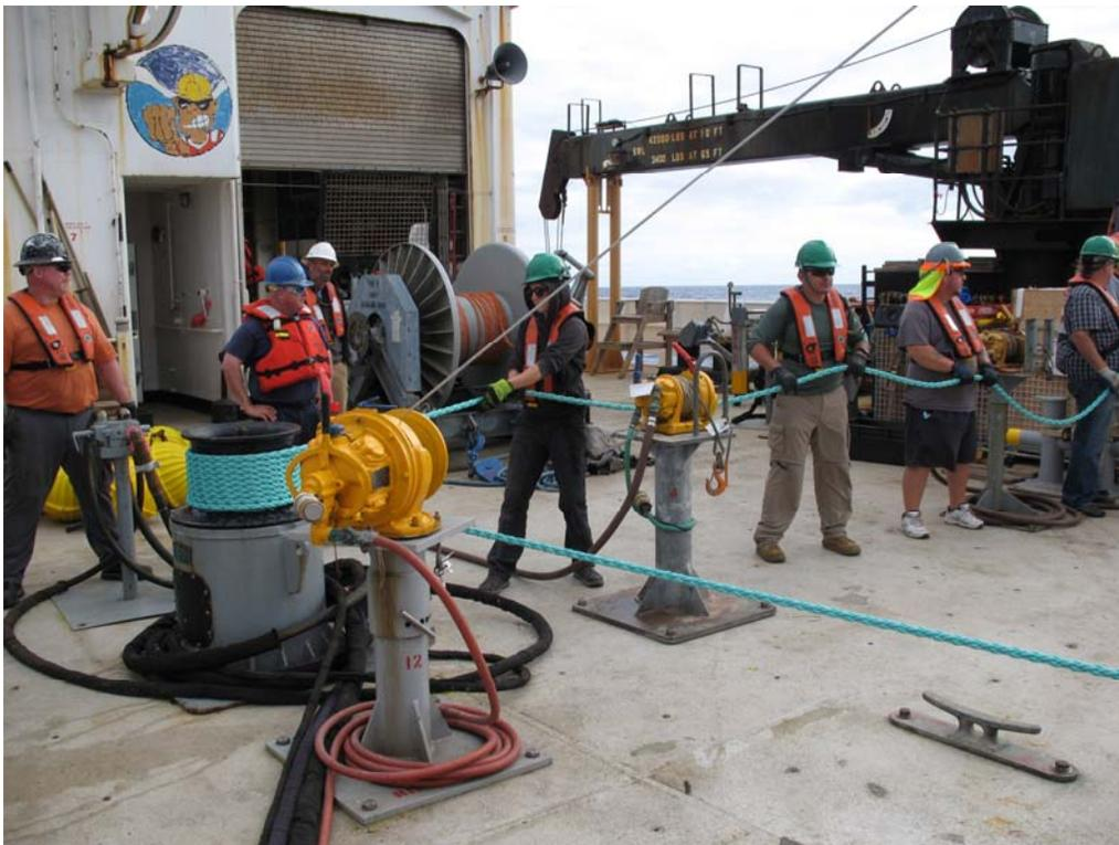
**Figure IV-2. Recovery of Colmega rope using capstan.**
