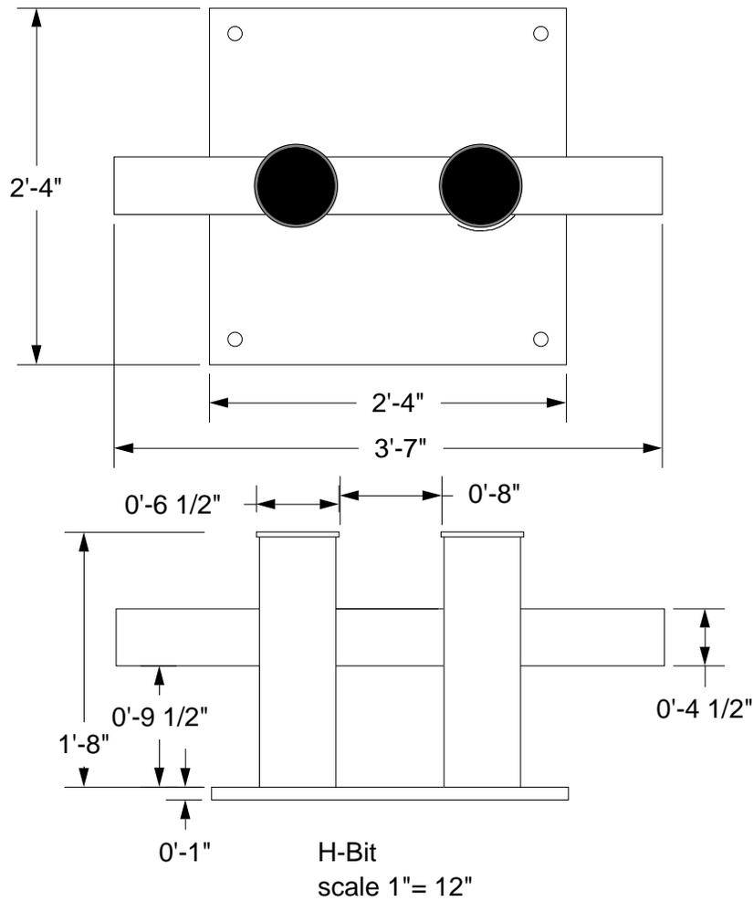
Figure 39: H-Bit winding for releasing the final 2000 m of line.
