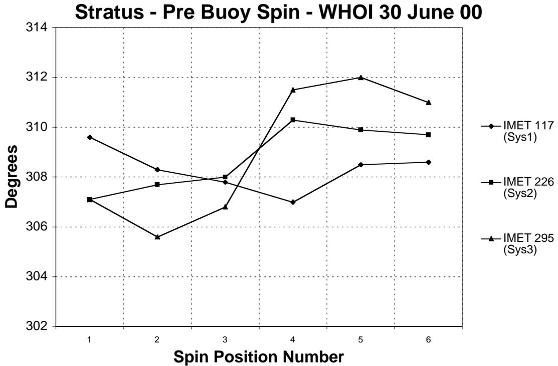
**Figure 6: Pre-deployment Buoy Spin at WHOI.**
