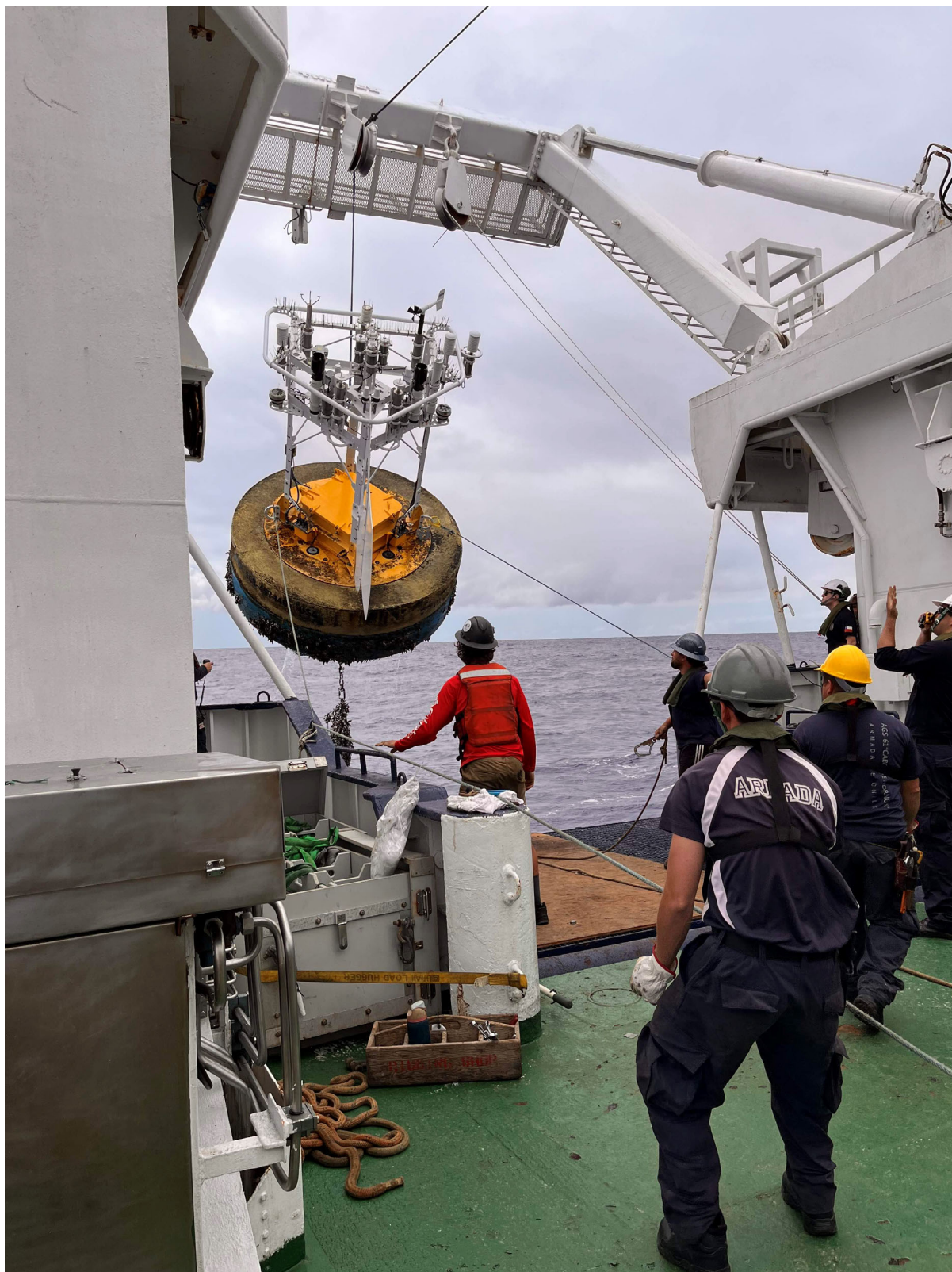
Figure IV-3. Stratus 22 buoy being recovered on March 18, 2025. Note missing outboard bracket on port (left) side of the buoy where standalone HRH and SBE39AT were installed at deployment
