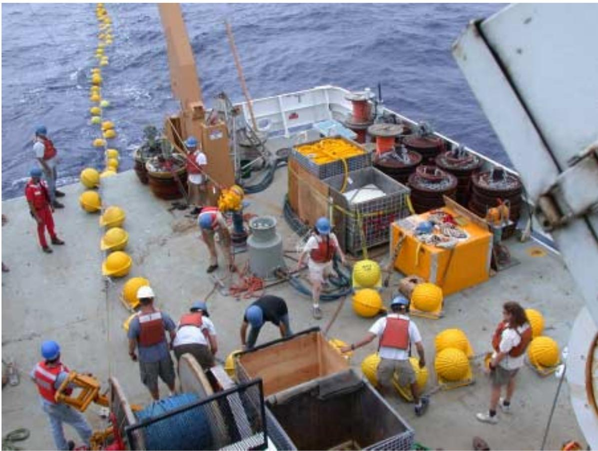
**Figure 74: Deployment of glass balls**
