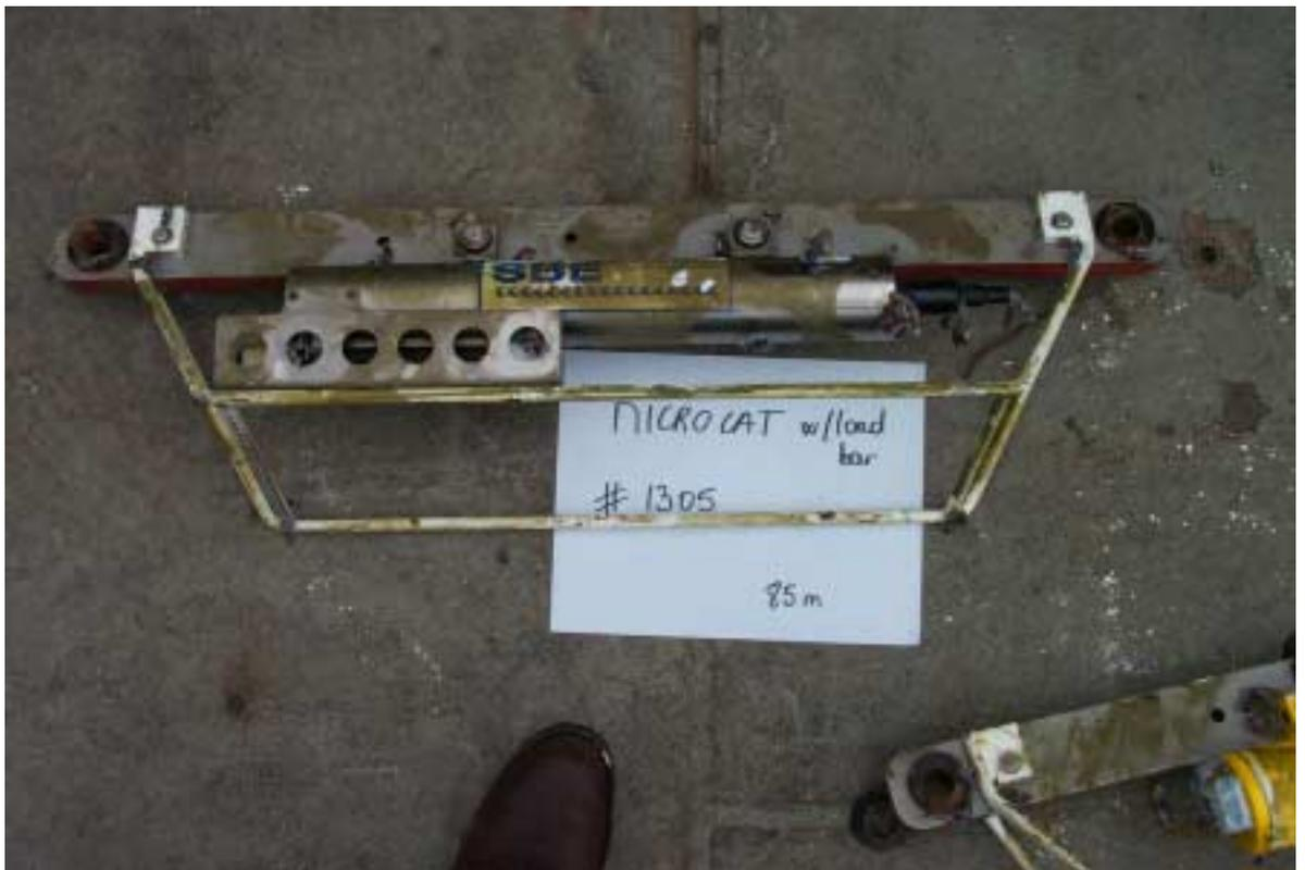
**Figure 35: MICROCAT instrument at 85 m depth.**
