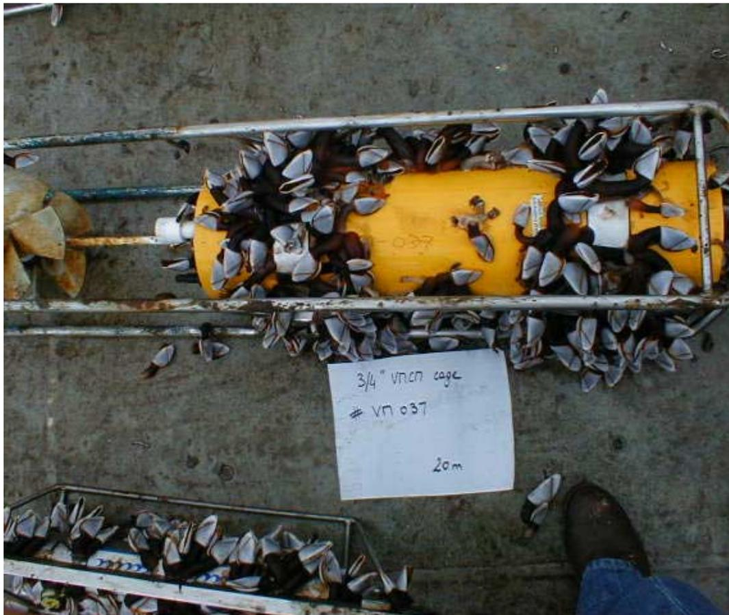
**Figure 36: VMCM instrument at 20 m depth.**
