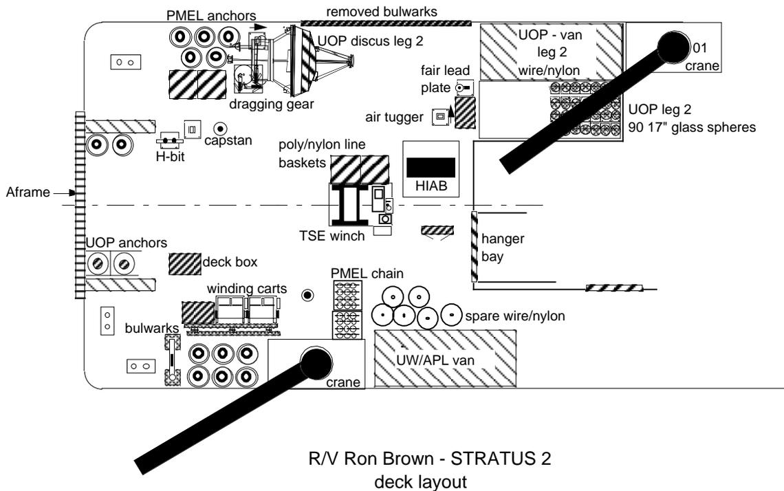
**Figure 69: Basic deck equipment and deck layout**
