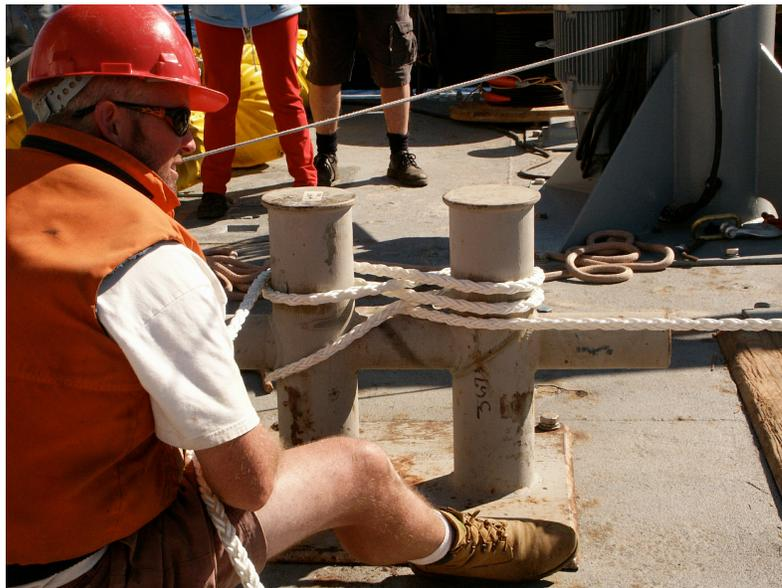
**Figure 15: H-Bit rigged for deploying 2000 meters of line.**
