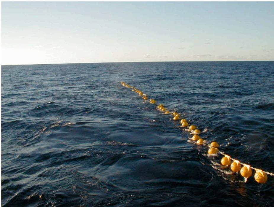
**Figure 16: Glass balls in hard hats deployed on mooring line.**
