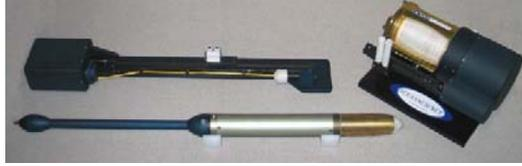
**Figure 7-2: Probe and Tail Spool, Re-winder & Winch**
