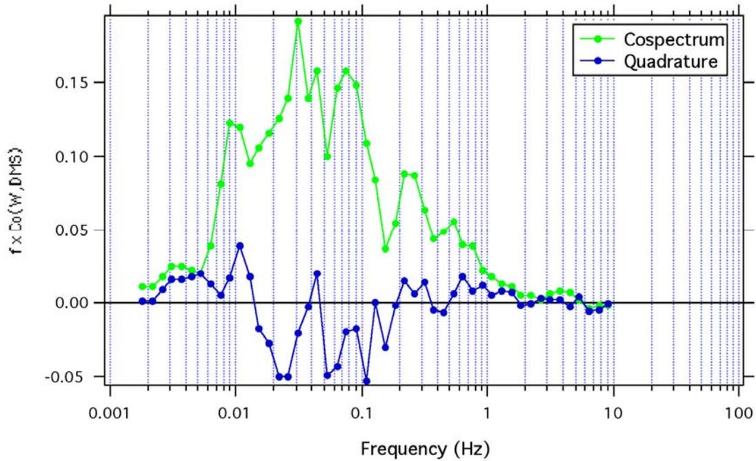
**Figure 10-2: A typical cospectrum between DMS and W, the motion-corrected vertical wind velocity. The sea-to-air flux of DMS was derived both from the direct covariance between DMS and W and also from the integral of the above spectrum. Most of the flux was found between 0.01 to 0.5 hz.**
