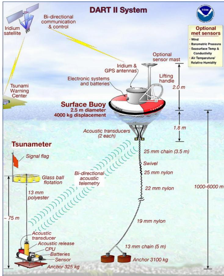
**Figure 6-1: Schematic of the DART mooring system**
