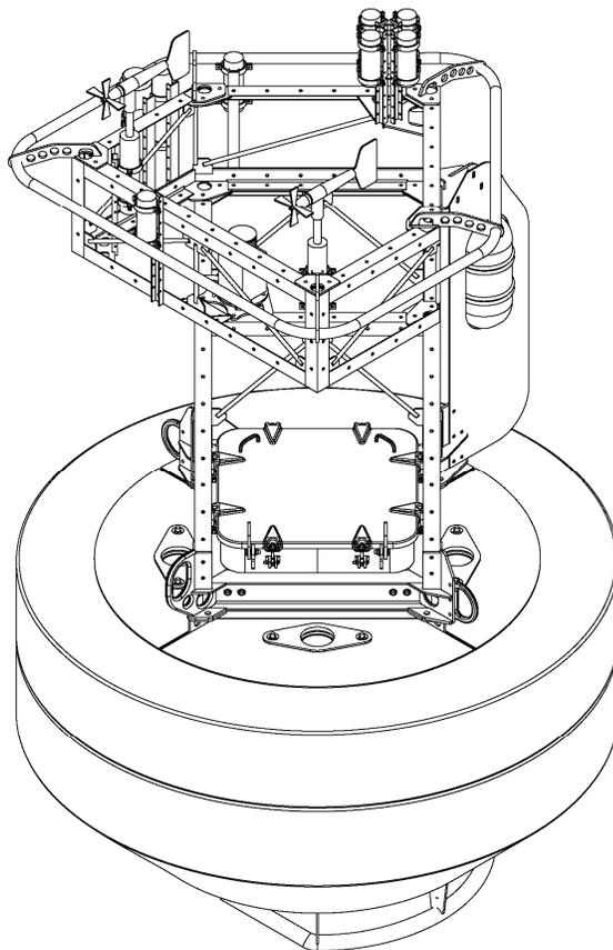
**Figure 3-1: Representation of Stratus 9 ASIMET buoy.**
