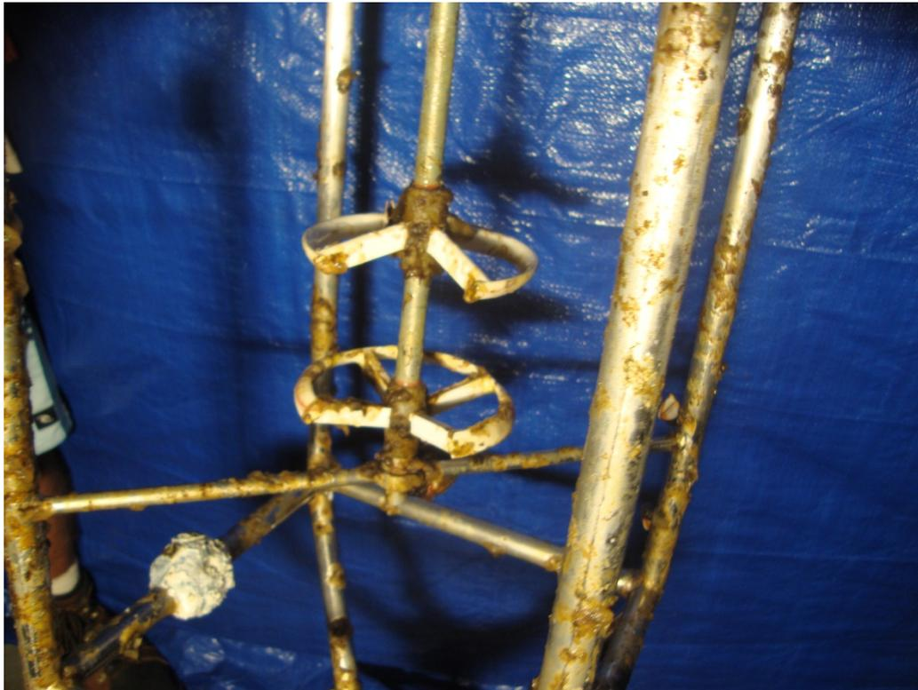
Figure C2. WHOTS-10 MAVS deployed at 20 m, after recovery.
