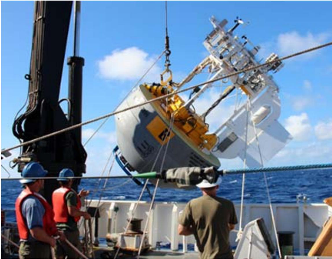
**Figure 11. WHOTS-11 buoy deployment. The buoy is lifted over the (non-removable) gunwales with the ship's crane. Tag lines for the crane whip, quick release, buoy deck, and buoy tower can be seen. The bolted on vane extension can also be seen in this photo.**
