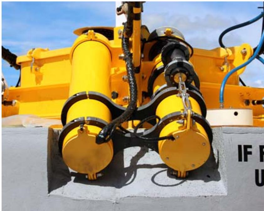
Figure 7. Remote line deployment system on the WHOTS-11 buoy.
