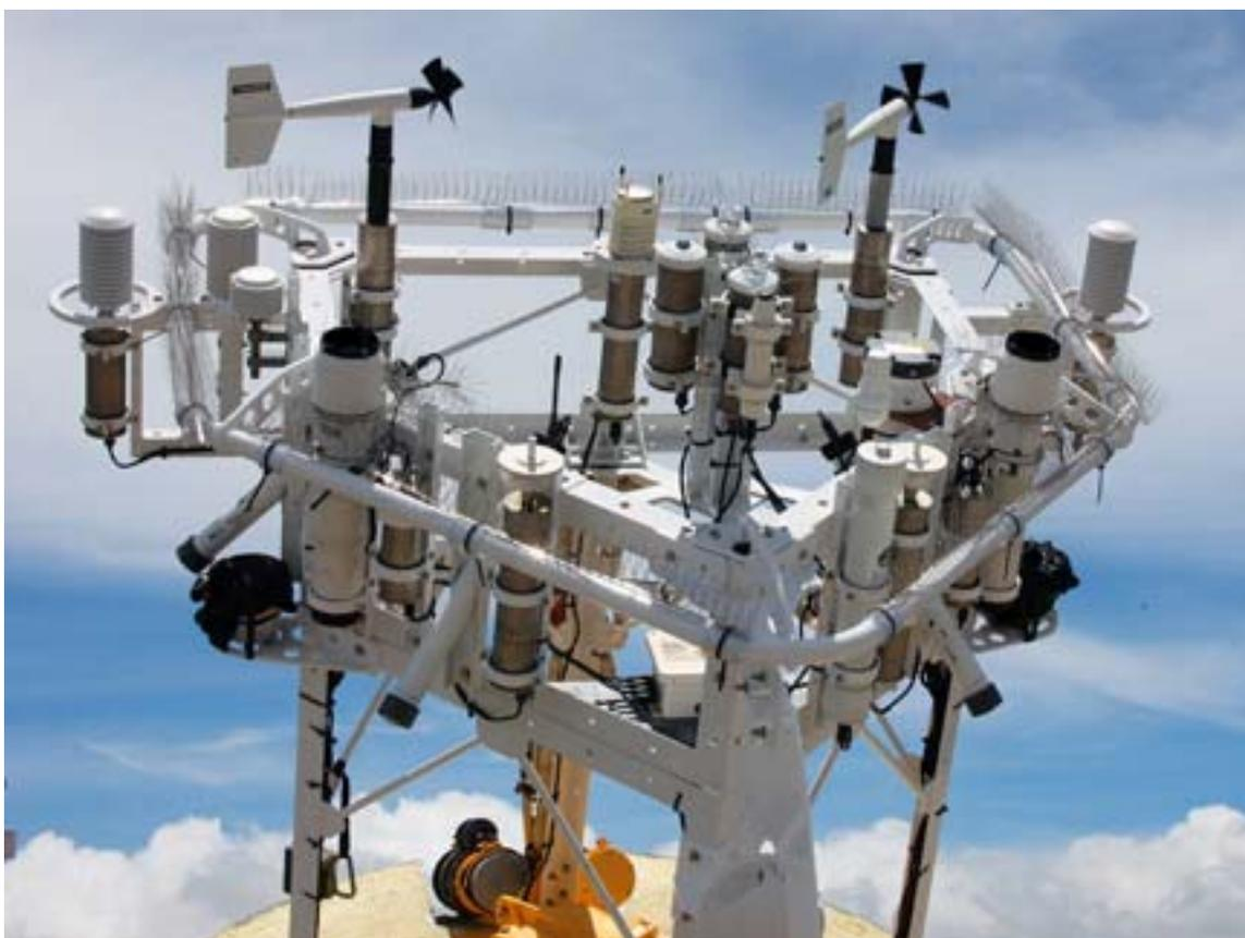
**Figure 8. WHOTS-11 tower top, showing the location of ASIMET modules and a variety of auxiliary sensors.**
