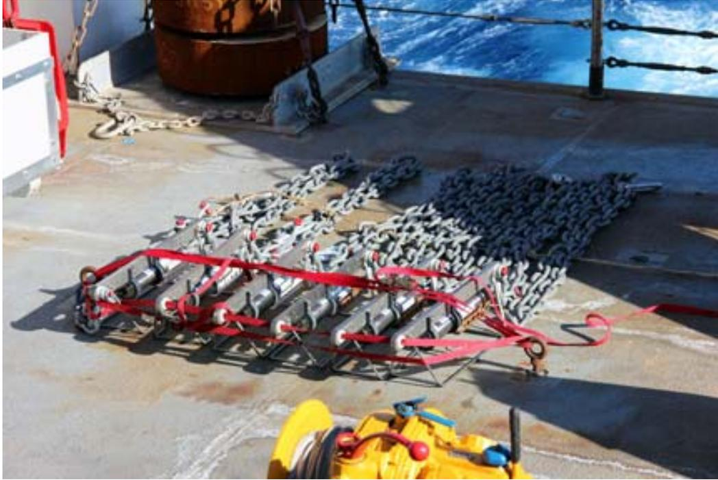
**Figure 10. Subsurface instrumentation assembled and laid out in sequence on deck prior to deployment. The deepest instrument is at the far left.**
