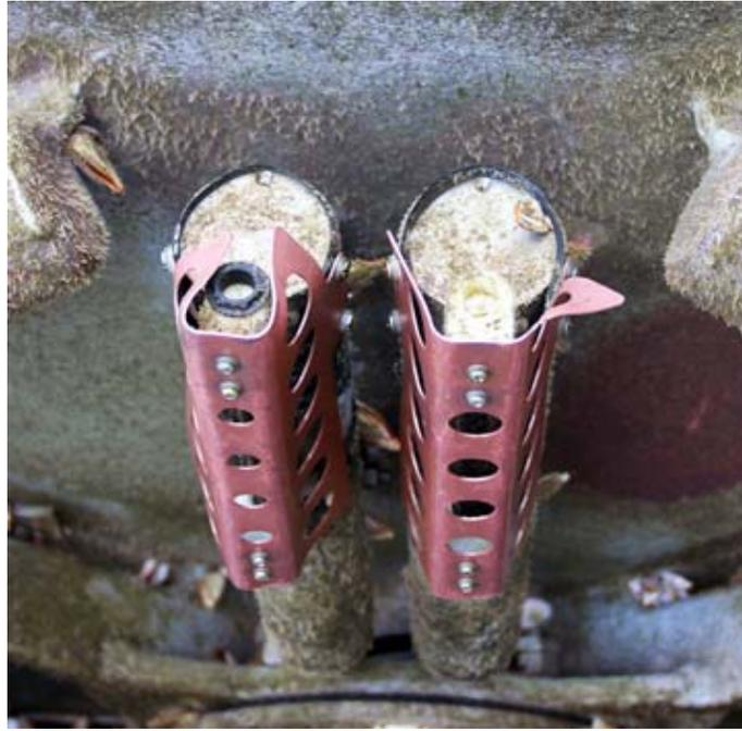
**Figure F3. WHOTS-10 buoy hull SBE-37 instruments.**
