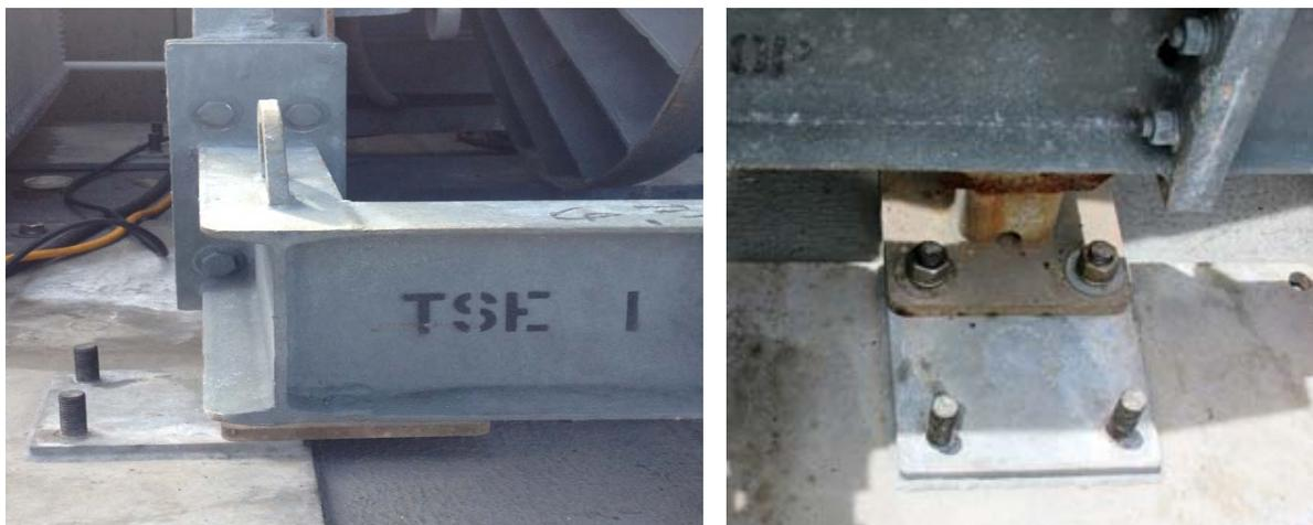
**Figure 2. TSE winch #1 fit to the deck of the *Hi'ialakai*. These photos show the port side aft corner with two of the four adapter plate studs mated to the foot of the winch.**
