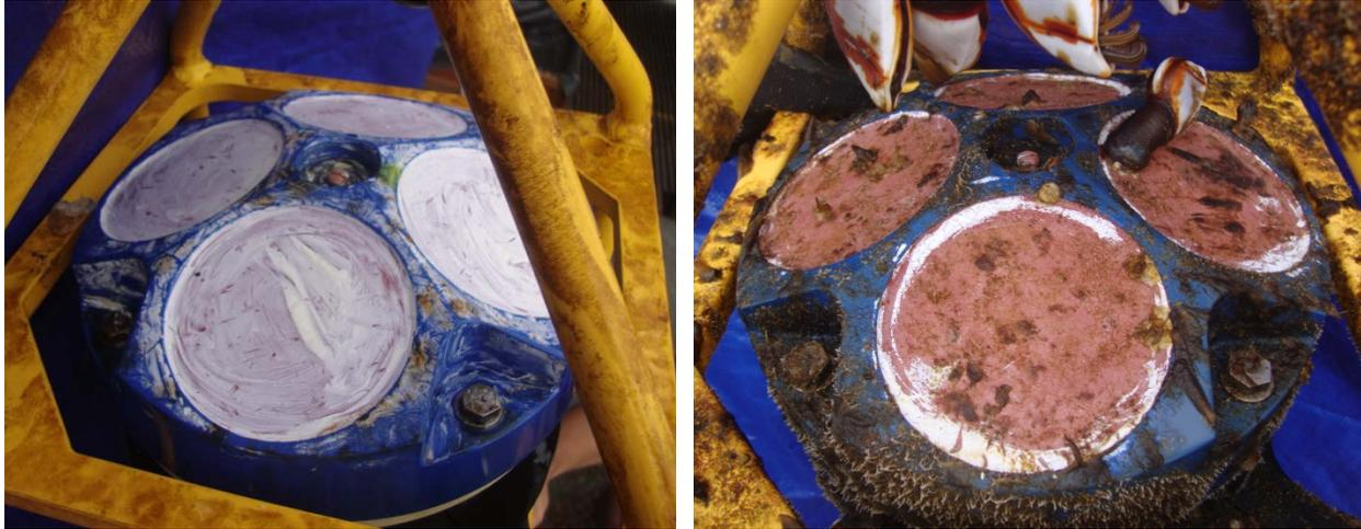
**Figure C1. WHOTS-10 ADCPs deployed at 125 m (left) and 47.5 m (right) after recovery.**
