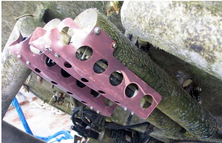
**Figure D1. WHOTS-8 buoy hull and SBE-37 instruments.**
