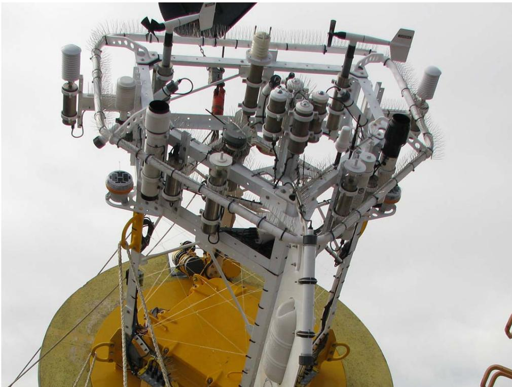
**Figure 8. WHOTS-9 tower top, showing the location of ASIMET modules. A SBE-39 (port side in front of PRC) supplemented the ASIMET HRH modules. A Vaisala WXT multi-parameter sensor was mounted between the two WND modules. A self-contained GPS module was mounted just forward of the starboard BPR.**
