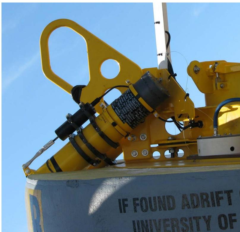
**Fig. 7. Remote line deployment system on the WHOTS-9 buoy.**
