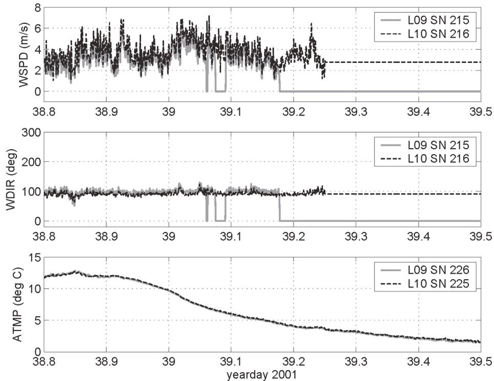
**Figure 5. Time series of wind speed (upper) and direction (middle) from two wind modules, SN 215 and 216, on the buoy in Charleston. Both wind sensors failed as the air temperature (lower) dropped below 5 deg C.**
