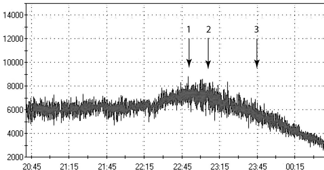
**Figure 11. Trawl winch tension vs. time during dragging operations, starting about 15 min after wire haul-back. Arrows indicate approximate times when (1) dragging weights were off the bottom, (2) release was fired and (3) release was at its minimum slant range.**
