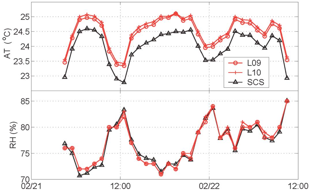
**Figure 33. Air temperature (AT, upper) and relative humidity (RH, lower) for the NTAS-4 buoy systems (L09, o and L10, +) and the *Brown* (x) during the intercomparison period.**
