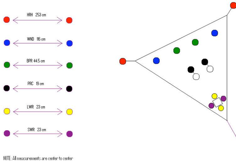
**Figure 18. NTAS-4 tower top layout and module separations shown graphically.**
