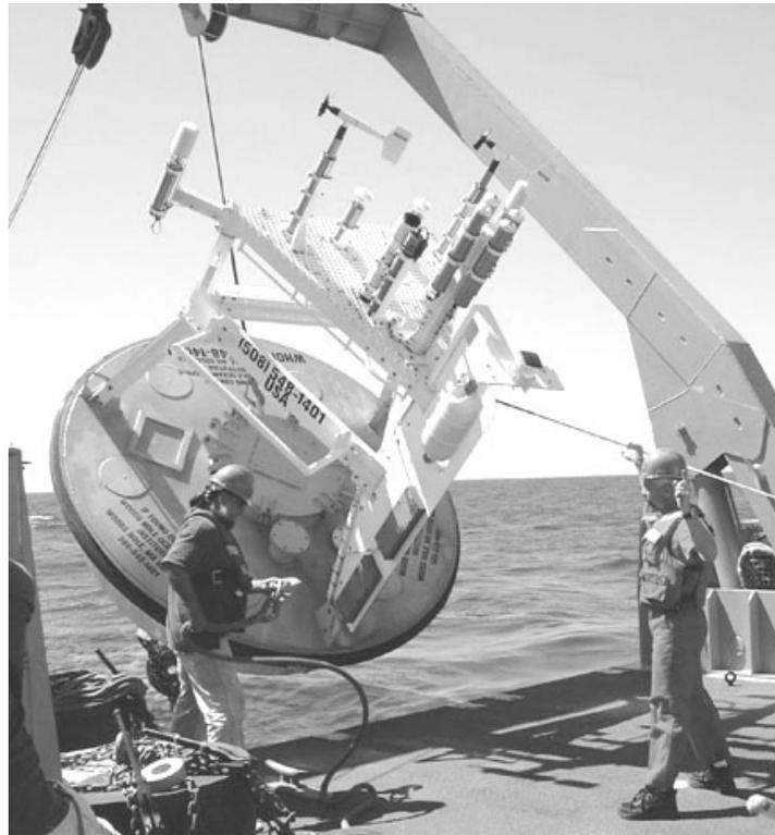
**Figure 7. NTAS-3 buoy being lifted through the A-Frame (Photo by Wade Blake).**
