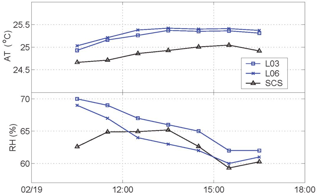
Figure 28. Air temperature (AT, upper) and relative humidity (RH, lower) for the NTAS-3 buoy systems (L03, o and L06, +) and the *Brown* (x) during the intercomparison period.
