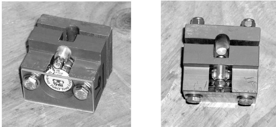
**Figure 23. Tidbit temperature logger in plastic bracket used for attachment to wire. Front view (left) and top view (right) are shown.**
