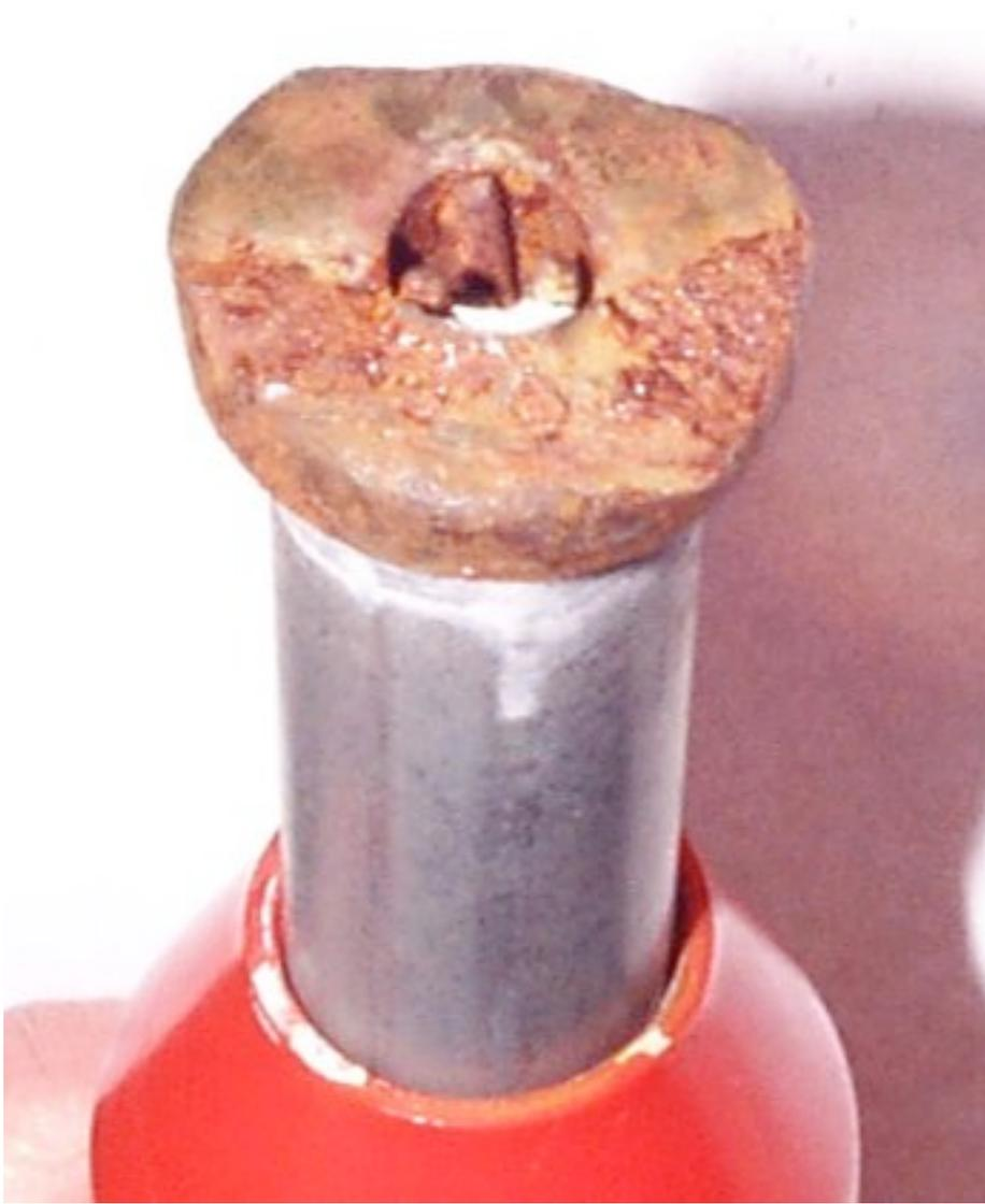
Photograph showing the fracture surface from the returned ½ inch swage socket.
