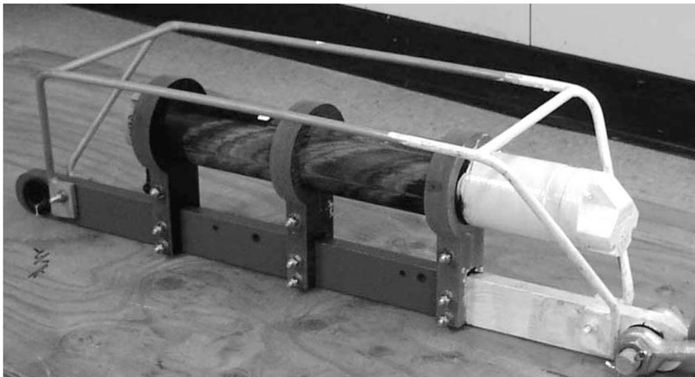
**Figure 19. The Aquadopp current meter attached to a titanium load bar and protected by a bolt-on cage. Anti-fouling paint has been applied to the upper portion of the assembly, including the transducer.**
