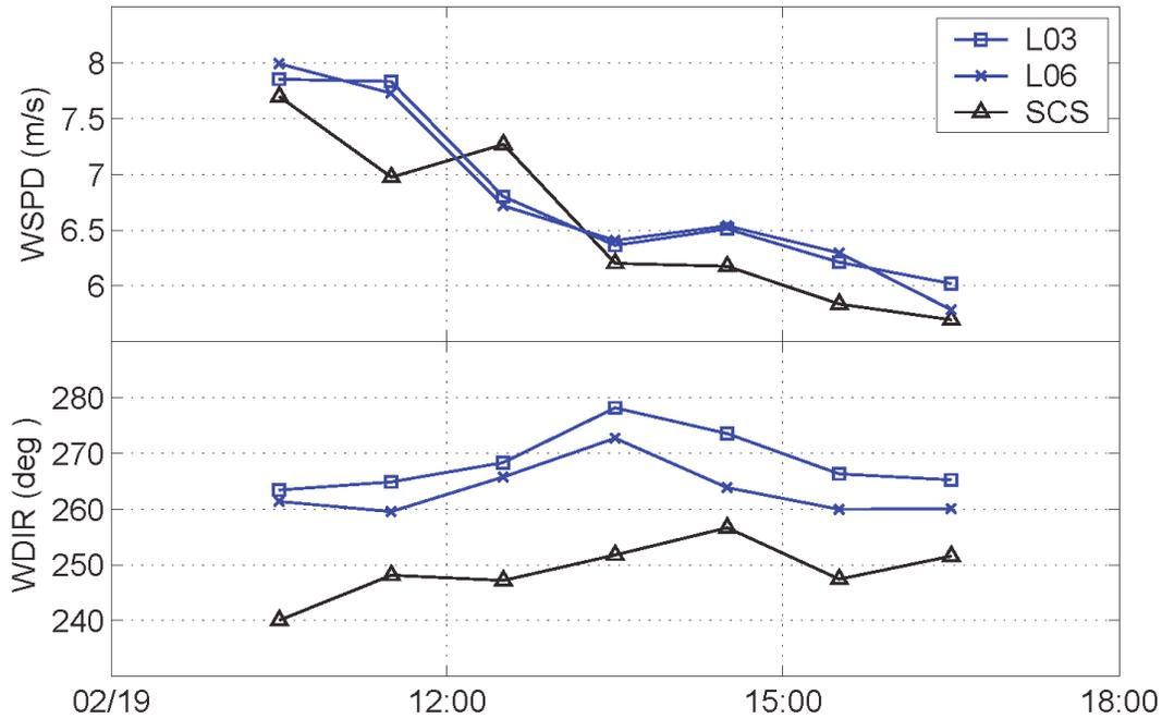
**Figure 32. Wind speed (WSPD, upper) and wind direction (WDIR, lower) for the NTAS-3 buoy systems and the *Brown* during the intercomparison period.**
