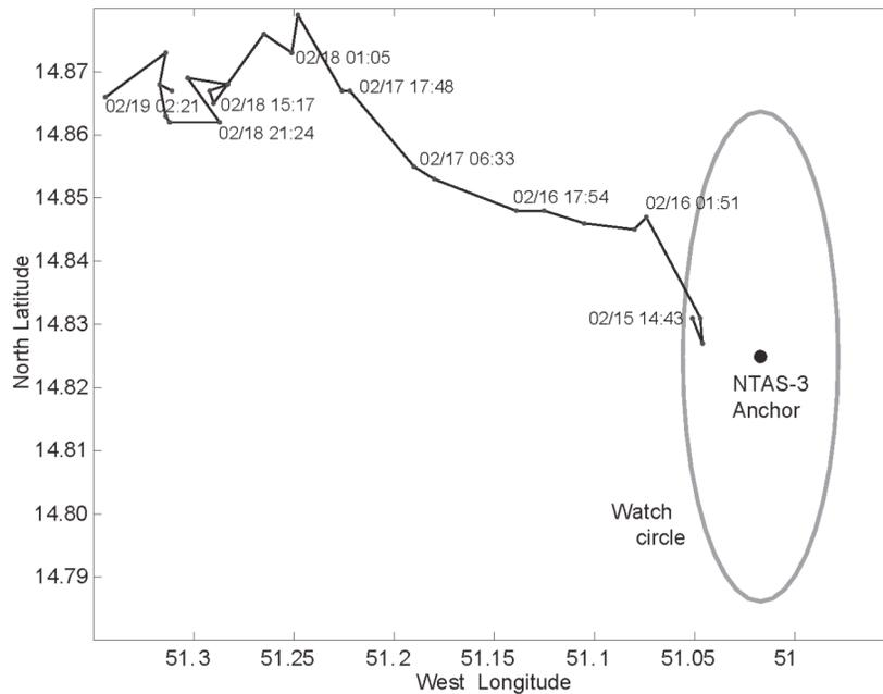
**Figure 6. NTAS-3 buoy drift track after mooring component failure on 15 February. The buoy was recovered on 19 February.**
