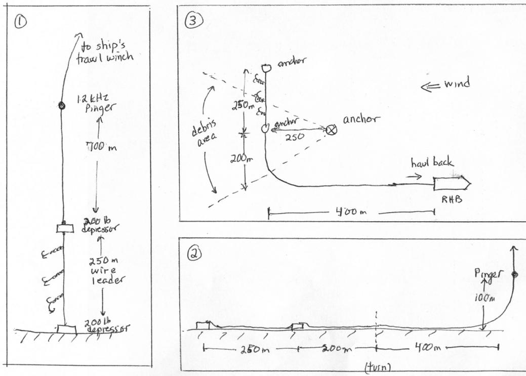
**Figure 9. Concept sketch for dragging operations. Dragging gear is attached to the ship's trawl wire (1), the lower 850 m of wire is laid out on the sea floor as (2), as the ship maneuvers in an L-shaped pattern (3).**
