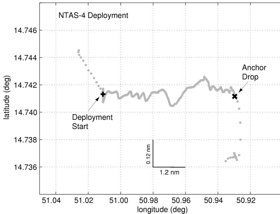
**Figure 25. Ship track during NTAS-4 deployment. The period shown includes the deployment start (+), the deployment approach, and the anchor drop (x). Dots are evenly spaced at 1 min intervals; larger dot separation indicates faster ship speed. Note that the vertical scale is exaggerated by a factor of 10 relative to the horizontal scale.**
