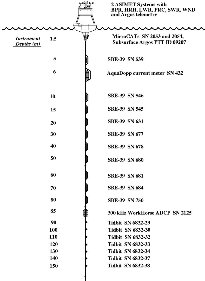
**Figure 15. NTAS-4 mooring detail in the upper 150 m.**
