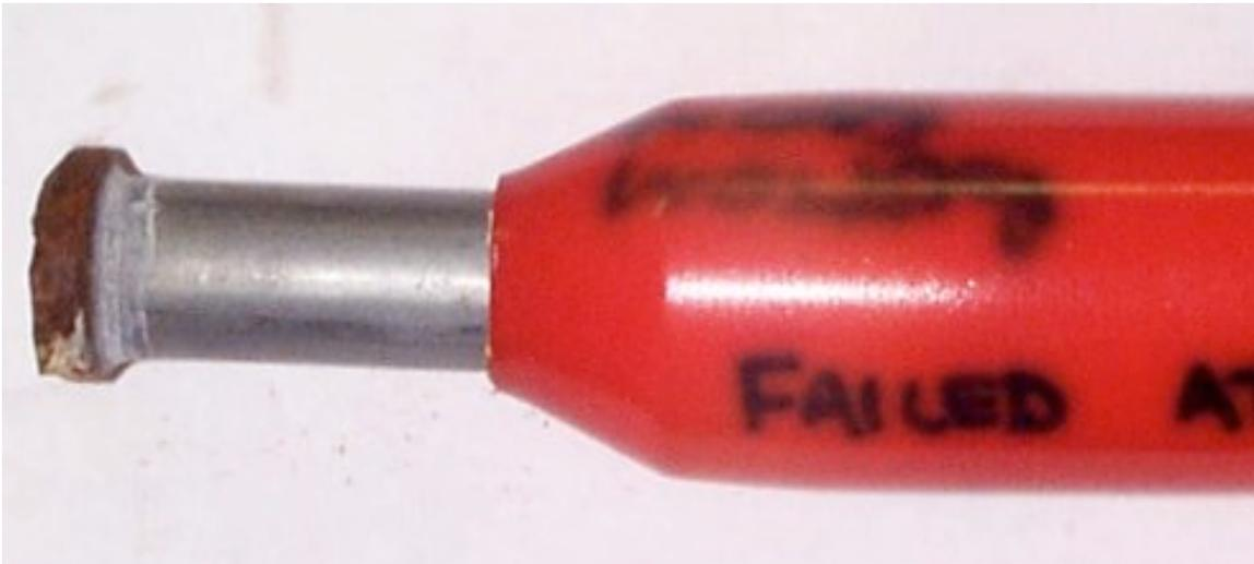
Figure 2. Photograph showing the shank section of the fractured swage socket.
