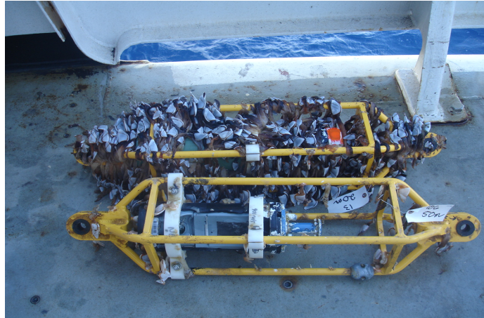
Figure 4-3a. RCM-11 recovered (back), SeaGuard crushed (foreground).
