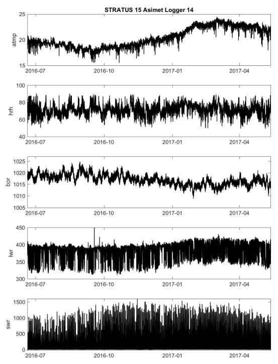
Figure IV-7. 1-minute data recovered from logger 14 (system 2) on Stratus 15: air temperature, air humidity, barometric pressure, incoming longwave radiation, incoming shortwave radiation
