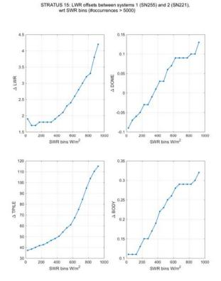
Figure IV-16. Offsets (median from all deployment) between longwave sensor on system 1 and 2 recovered from Stratus 15 as a function of concomitant shortwave radiation also measured on Stratus 15.
