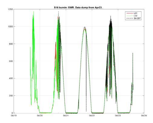
Figure II-7. Stratus 16 burn-in data from April 23 2017 download: shortwave radiation (SWR) in W m<sup>-2</sup>. Figure II-8. Stratus 16 burn-in data from April 23 2017 download: longwave radiation (LWR) in W m<sup>-2</sup>.
