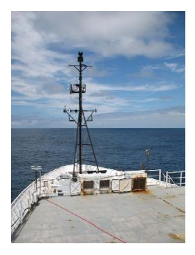
Figure III-12. PSD and ship sensors on bow mast; PSD radiation sensors on port side of 02 deck.
