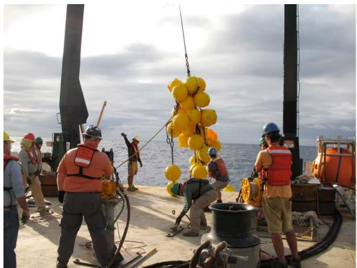
Figure IV-1. Recovery of glass balls from Stratus 15 mooring.
