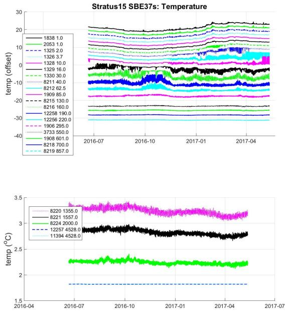
Figure IV-11. Temperature data (with offset for readability) from SBE37s recovered from Stratus 15. Legend indicates serial number and nominal depth of each instrument.
