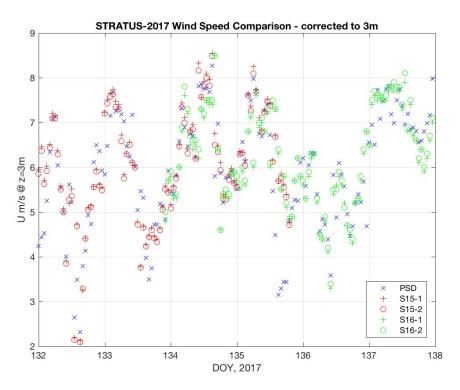
Figure III-17. Time-series of wind speed adjusted to 3 m from NOAA ESRL (PSD), ship (SCS) and Stratus 15 and 16 ASIMET systems 1 and 2, from May 12 to 17 2017.
