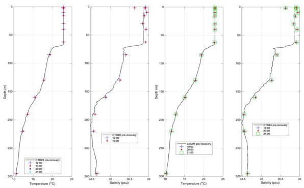
Figure III-32. Temperature and salinity profiles from CTD casts 3 (left) and 4 (right) made on May 14 2017 near Stratus 15 mooring, prior to its recovery. Colored symbols denote concomitant data from SBE37 instruments mounted on Stratus 15.
