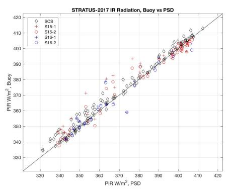
Figure III-28. Scatter plot of longwave incoming radiation from NOAA ESRL (PSD), versus ship (SCS) and Stratus 15 and 16 ASIMET systems 1 and 2, during inter-comparisons.
