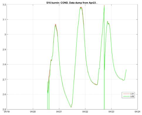
Figure II-10. Stratus 16 burn-in data from April 23 2017 download: conductivity (COND) in S m<sup>-1</sup>.
