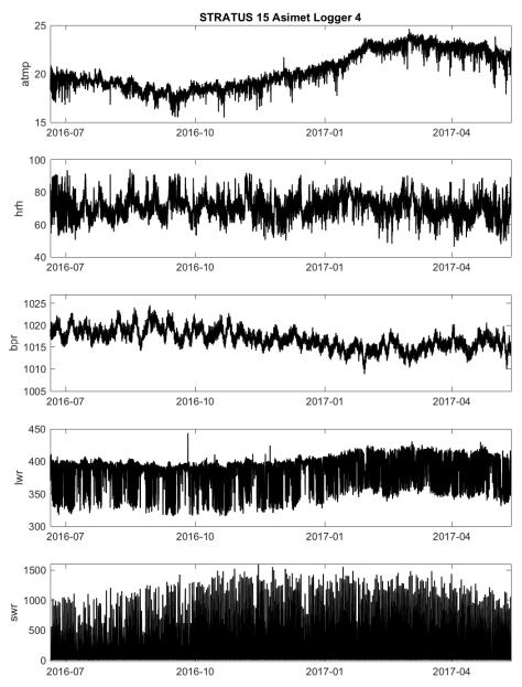
Figure IV-6. 1-minute data recovered from logger 4 (system 1) on Stratus 15: air temperature, air humidity, barometric pressure, incoming longwave radiation, incoming shortwave radiation
