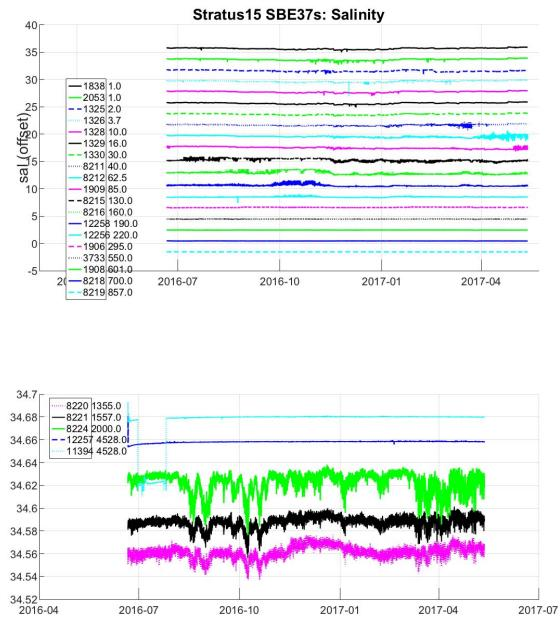
Figure IV-10. Salinity data (with offset for readability) from SBE37s recovered from Stratus 15. Legend indicates serial number and nominal depth of each instrument.
