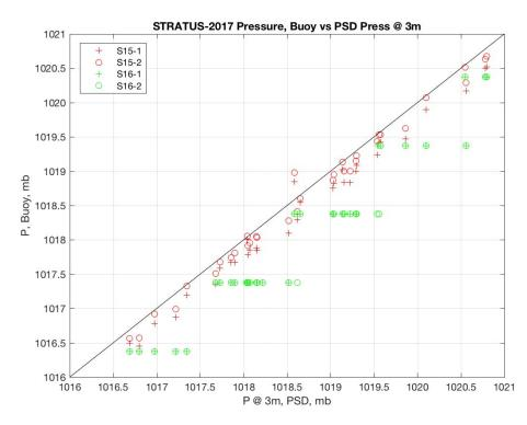
Figure III-30. Scatter plot of barometric pressure adjusted to 3 m from NOAA ESRL (PSD), versus ship (SCS) and Stratus 15 and 16 ASIMET systems 1 and 2, during inter-comparisons.
