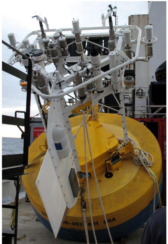
Figure III-1. Stratus 16 prior to deployment: buoy and meteorological tower.
