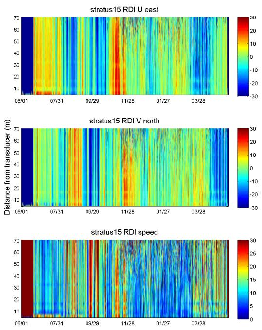
Figure IV-14. Current data from RDI Workhorse ADCP recovered from Stratus 15.
