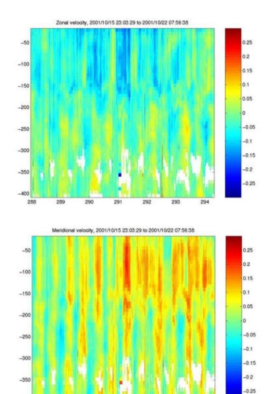
Figure 64: Zonal and Meridional Currents velocity for the shipboard ADCP.
