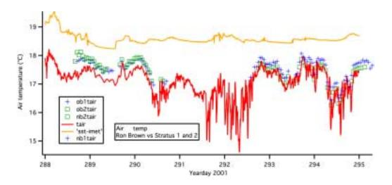
Figure 46: Comparison of buoy air temperatures (°C) from Stratus 1 (left) and 2 (right) buoys with ship and ETL data. For reference, IMET SST, which is  $\sim$ 1° warmer is shown.
