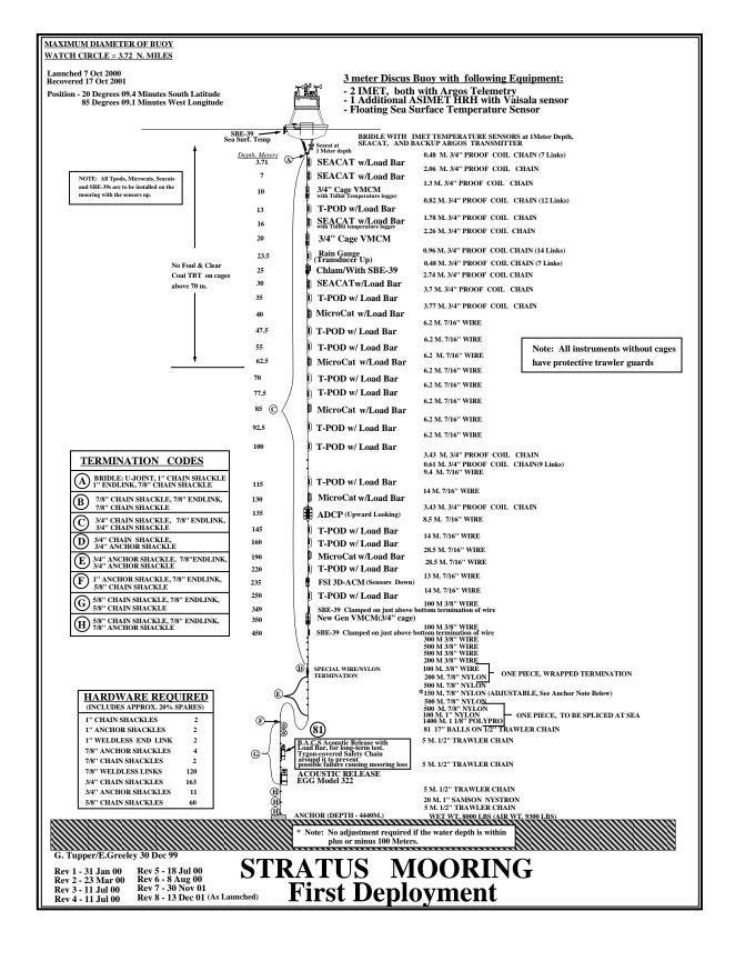
Figure 31: Stratus 1 mooring diagram – recovery.
