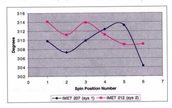
Figure 40: Pre-deployment Buoy spin at WHOI.
