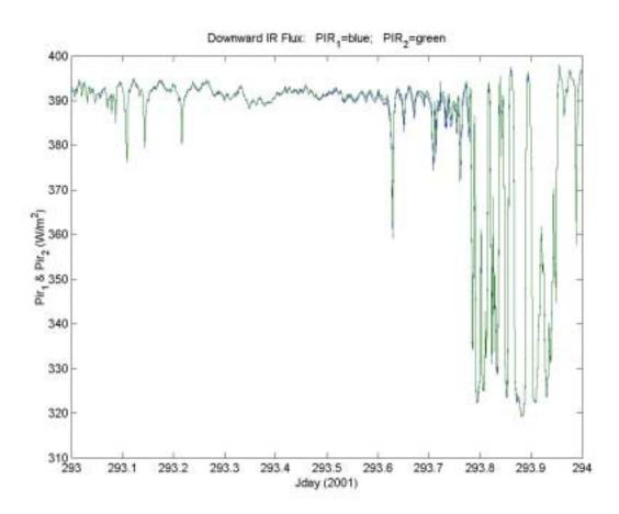
Figure 12: Time series of downward infrared radiative flux.
