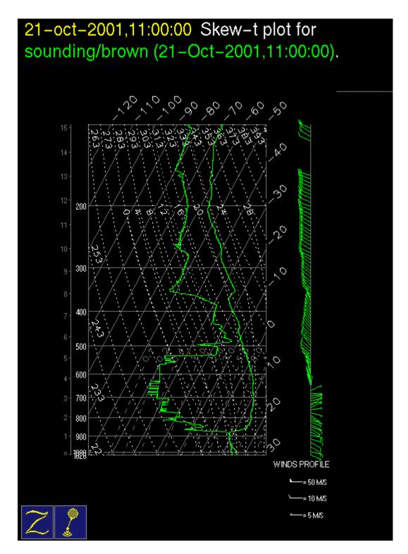
Figure 23: Upper-air sounding launched at 11 UTC October 21 (Day 294). No quality control has been applied. Dew point is curve to left and temperature is curve to left.
