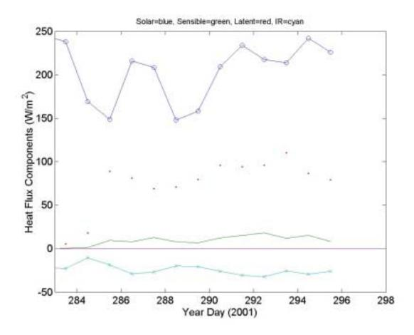
Figure 18: Time series of daily – averaged flux components: solar radiative flux (dashed blue), net infrared radiative flux (cyan x), sensible heat flux (green solid), and latent heat flux (red dots).
