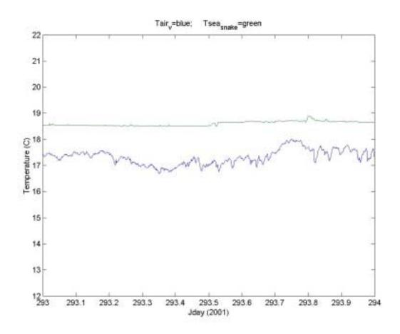
Figure 14: Time series of ocean temperature. Blue line is 5 – meter depth ship thermosalinograph intake, green dots are the ETL seasnake (approximately 5 – cm depth).
