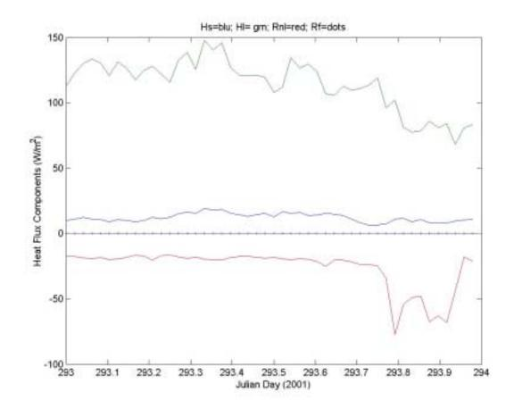
Figure 13: Time series of surface net heat flux components in meteorological coordinates. Sensible, latent, net infrared (downwelling minus upwelling), and rain.
