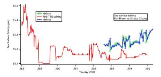
Figure 52: Comparison of Sea Surface Salinity (psu) from the two IMET systems on the Stratus 2 buoy with ship TSG data.
