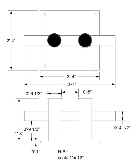
Figure 72: H-Bit winding for releasing the final 2000 m of line.
