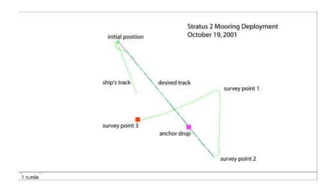
Figure 5: Target track path (black line) and ship's track (green) recorded by GPS during the mooring deployment, the acoustic survey of the anchor position, and the subsequent occupation of a position 1/4 mile downwind of the surface buoy.
