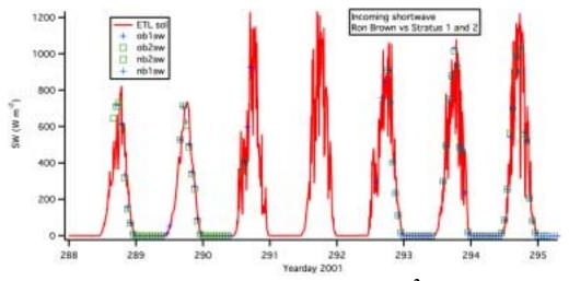
Figure 49: Comparison of incoming short-wave (W/m²) from the two IMET systems on the Stratus 1 (left) and 2 (right) buoys with ETL data.
