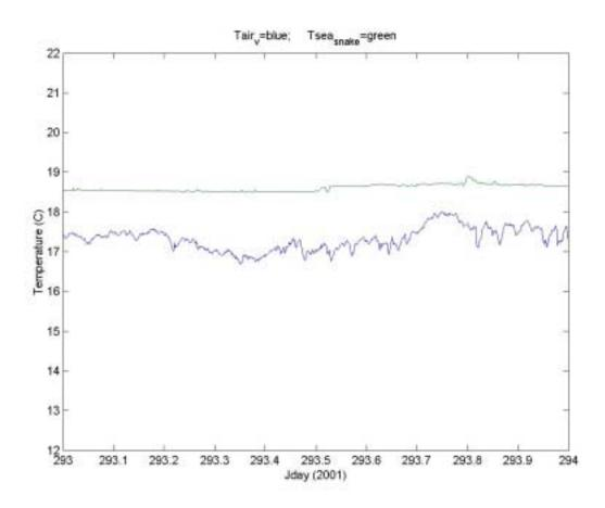
Figure 9: Time series of near – surface ocean temperature and  $15\ m$  air temperature.
