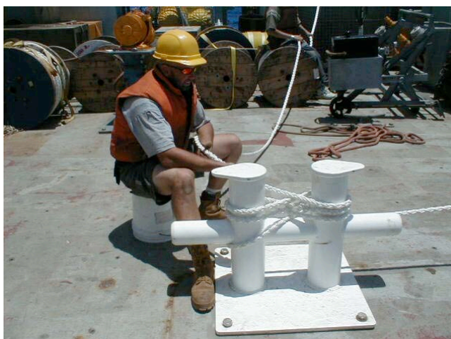
Figure 13. H-Bit Rigged For Deploying 2000 Meters Of Line.
