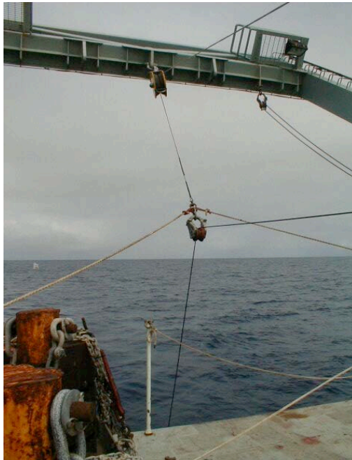
Figure 12. Using The Hanging Block To Control Deployment.
