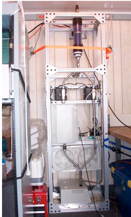
Figure 45. The APS and furnace set up used in the data collection.
