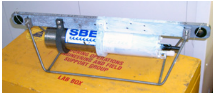
Figure 3: An SBE-16 (SeaCat) painted with white anti-foulant
