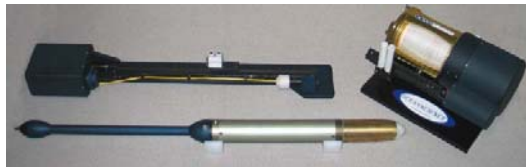
Figure 50: Probe/ Tail Spool, Re-winder & Winch
