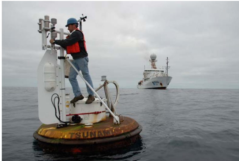
Figure 79: Service of SHOA DART buoy.
