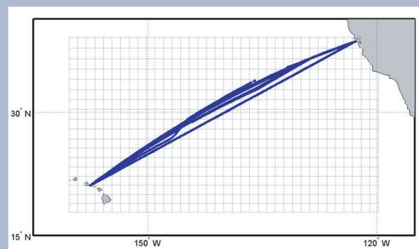
Ship tracks for the Honolulu to Oakland transects are shown along with ECMWF grid cells. The transects are along similar, but not identical, routes covering a distance of about 2400 miles. A typical transect passes through 34 ECMWF grid cells. VOS data are averaged within each cell and compared to the matching ECMWF variables as a function of distance along the track. The 29 available transits provide about 1000 VOS/ECMWF comparisons.
