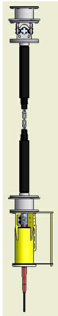
member. The chain is passed through a close-fitting reinforced hose, which is sealed at one end and filled with flexible polyurethane. An eight conductor, insulated "coil cord" is then wound over the chain/hose assembly, another reinforced hose is fed over this assembly, the chain is secured to flanges at each end, and the outer hose is filled with polyurethane. The result is a robust, yet compliant electro-mechanical section that brings protected conductors through the sea-surface interface.
