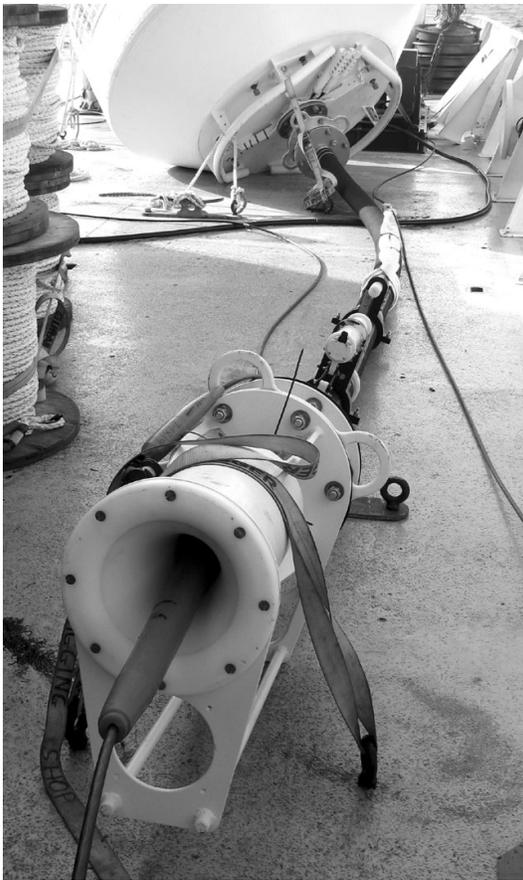
Once proper functioning of inductive communications is confirmed, the EM interface is assembled mechanically. During deployment, a portion of the mooring wire, with instruments attached, is run to the stern and the lower portion of the EM interface is lifted over the rail with a crane. The EM interface is then tied off until the buoy is ready to be lifted into the water.
