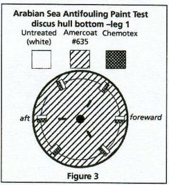
Chemotex is a calcium sulfonate based paint that the formulators found to work well as an ablative antifoulant. Field immersion tests<sup>1</sup> done in Woods Hole found that this coating seemed to minimize the growth of barnacles.
